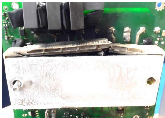
Fig. 1. Effect from swell voltage resulting in the damages of Electronic devices
