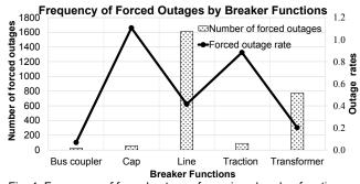
Fig. 4: Frequency of forced outages for various breaker functions.
