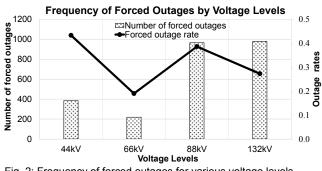
Fig. 2: Frequency of forced outages for various voltage levels.
