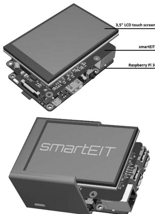
Fig. 7. The Smart EIT device.
