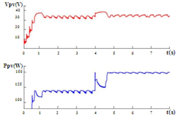
Fig.8. voltage and power characteristics under different irradiance .
