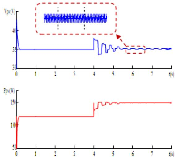
Fig.13. Shape of voltage and power front a variation of irradiance.
