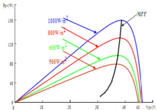
Fig.2. Changing the MPP during solar irradiance variations.
