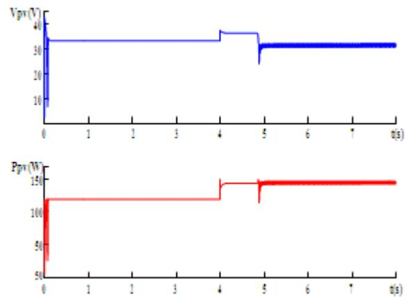
Fig.11.voltage and power face a variation of irradiance .
