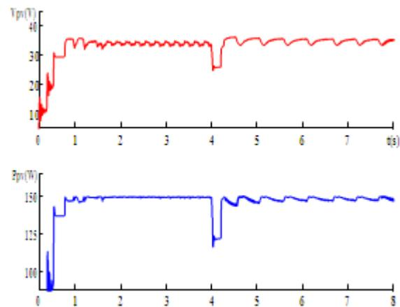
Fig.9. shape voltage and power against a variation of load
