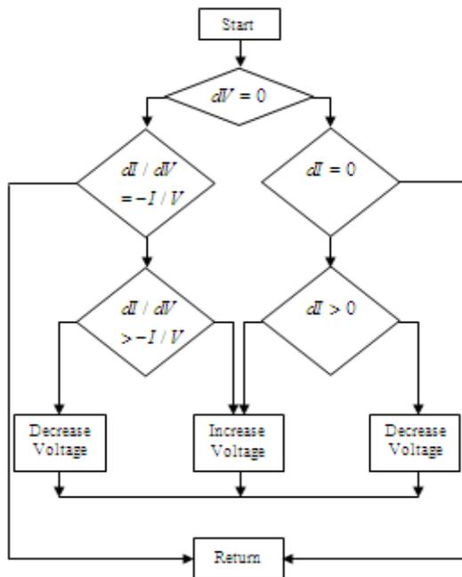
Figure 10. Increment Conductance
