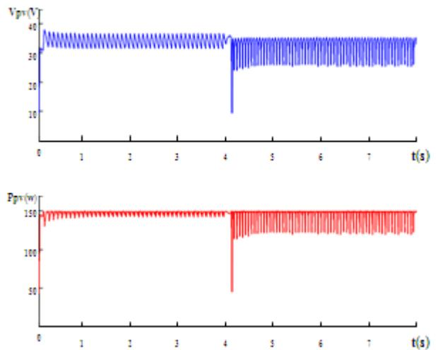
Fig.12 allure of vovltage and power facing a load variation.
