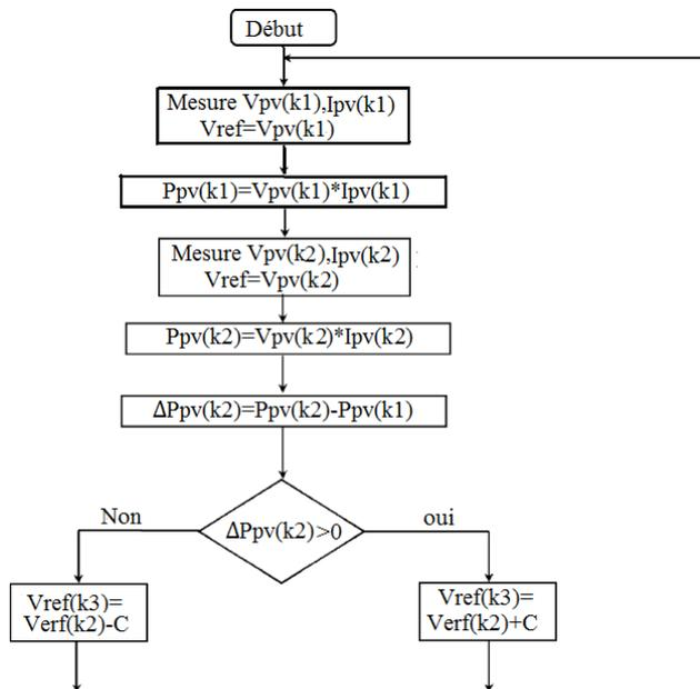
Fig.7. P&O Algorithm global structure
