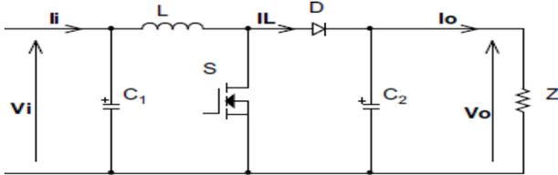
Fig.6. DC/DC boost converter
