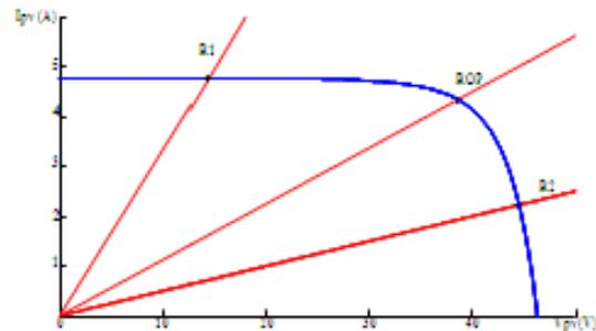
Fig.4. Influence of the load on the MPP
