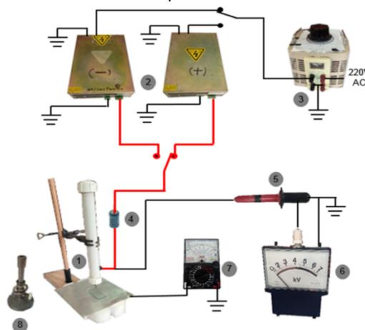
Fig. 1. Experimental setup. (1) Tip-plane configuration, (2) two high-voltage DC power supplies with negative and positive polarity, (3) Autotransformer, (4) Resistor of 8 M $\Omega$ , (5) Probe, (6) Electrostatic voltmeter, (7) Micro-ammeter, (8) Bunsen burner.
