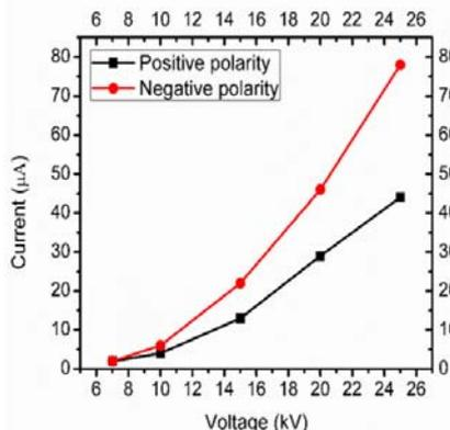
Fig. 2. Current - voltage characteristic of the power supply for negative and positive polarity
