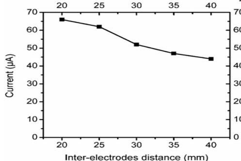
Fig. 12. Electrical discharge current evolution versus the interelectrodes distance. Corona Voltage = 25 kV, Negative polarity.
