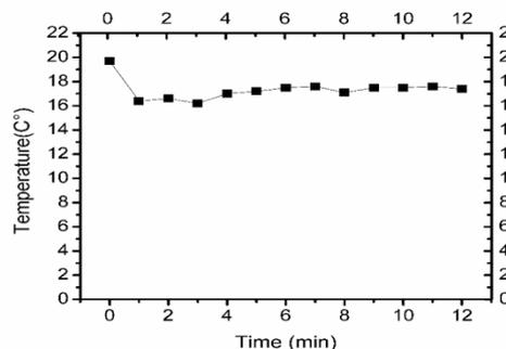
Fig.6. Characteristic of temperature effect on the load Corona Voltage = 25 kV, Interelectrode distance = 30 mm.
