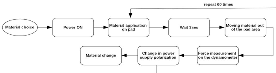
Fig. 1. Diagram of the measuring system.
