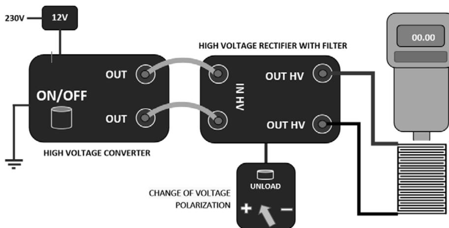
Fig. 2. Block diagram of pull-off force measurements.
