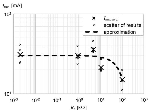
Fig. 7. Dependence of the maximum current value  $I_{\max \text{ avg}}$  on the additional resistance  $R_d$
