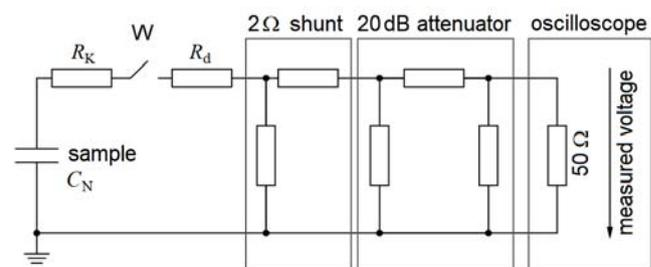
Fig. 1. The equivalent scheme of the measuring system for logging the discharge current-time characteristic during sample discharge, W – switch representing the occurrence of discharge (when closed)
