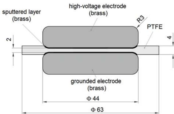
Fig. 2. Model of the reference capacitor
