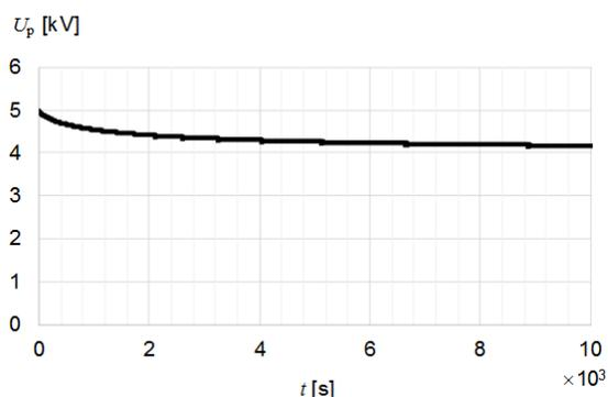
Fig. 5. Voltage-decay characteristic for reference capacitor
