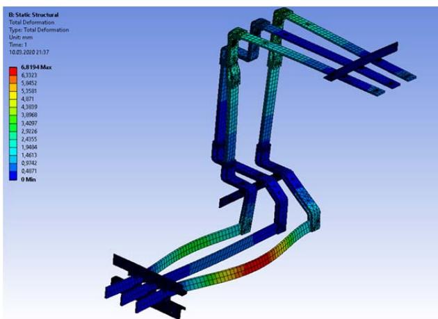
Fig. 3. The total stresses caused by the flow of the short-circuit current.
