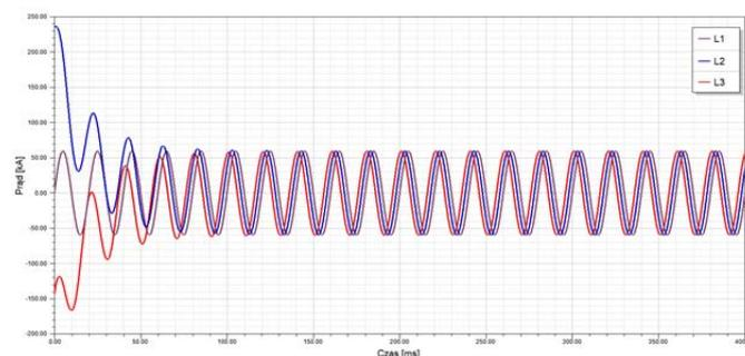
Fig. 4. Waveforms of three-phase short-circuit current.
