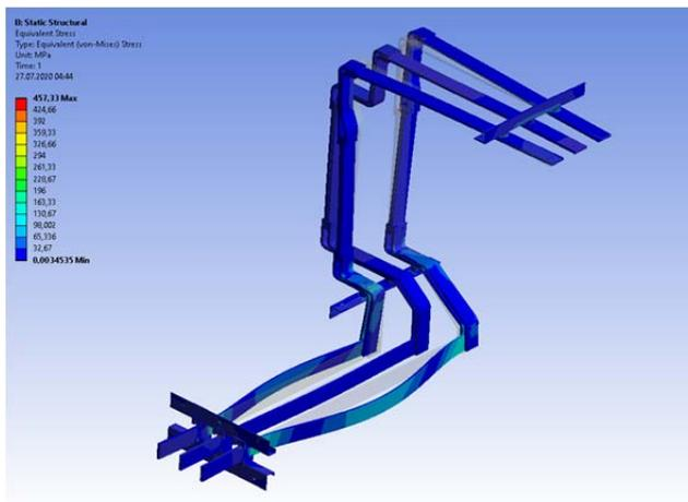
Fig. 2. Reduced stresses resulting from the flow of short-circuit current.
