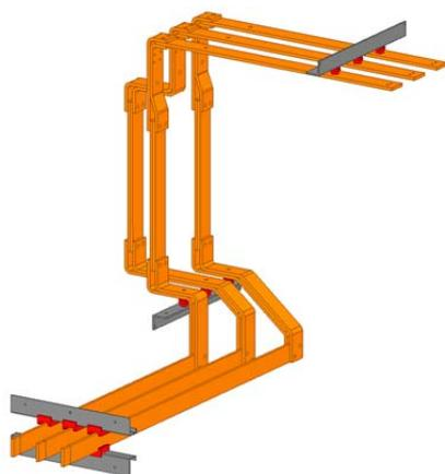
Fig. 1. Busbar model made in the SolidWorks program (cross-section of a single 60 x 10 mm busbar).
