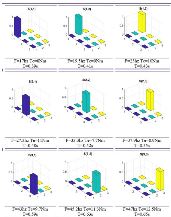
Fig 10. Test results for nine switch faults with different operation modes.
