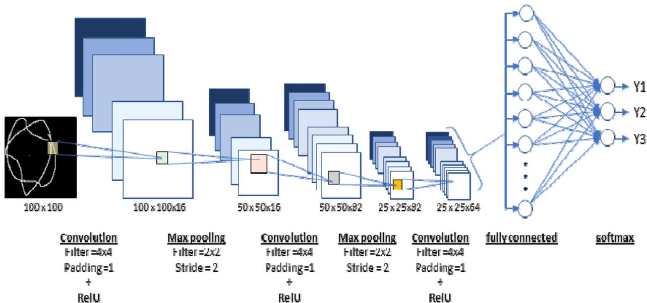
Fig.7. CNN architecture includes an input layer, convolutional layers and a softmax-type output layer.
