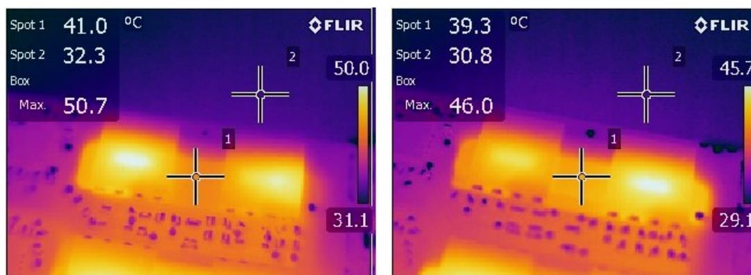
Fig.4. Thermal camera picture of FR4 based PCB – copper inlay (right), optimized thermal vias (left). Spot no.2 represents the heatsink temperature
