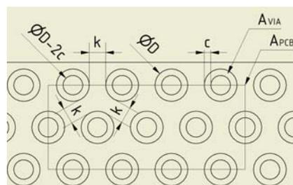
Fig.3. Parameters of printed circuit board thermal vias (top view)
