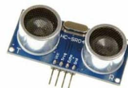
Fig. 2. The additional module HC-SR04
