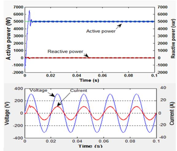
Fig.6. Powers, and single phase current / voltage (PF=1)
