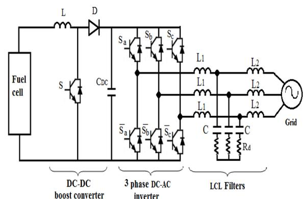
Fig.1. Proposed fuel cell grid connected system
