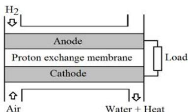
Fig.2. PEM fuel cell principle
