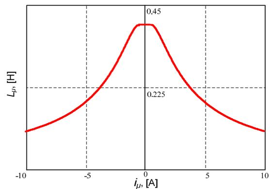
Fig. 3. The magnetizing inductance dependence on the magnetizing current
