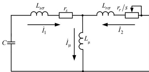
Fig. 2. IG equivalent circuit
