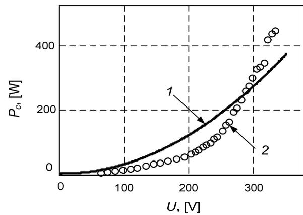
Fig. 1. Comparison of steel loss curves: 1 – curve obtained using the classical method [7], 2 – experimental curve
