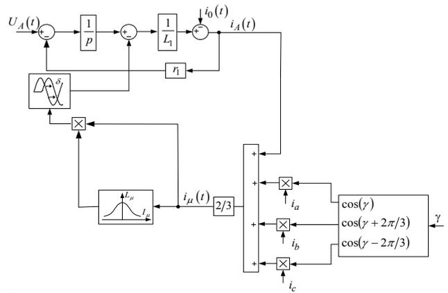
Fig. 4. IM stator phase block diagram taking into account the magnetic lag angle
