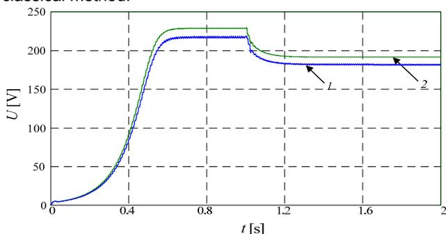
Fig. 6. The dynamic characteristics of IG with various methods of accounting for steel losses: 1 – according to expression (11), 2 – using the classical method
