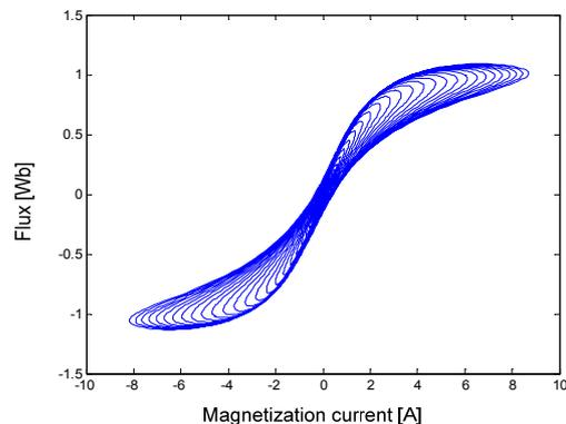
Fig. 5. Calculated hysteresis loops for self-excitation of an autonomous IG
