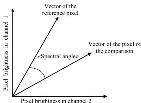
Fig. 3. Illustration of the classification by spectral angle method
