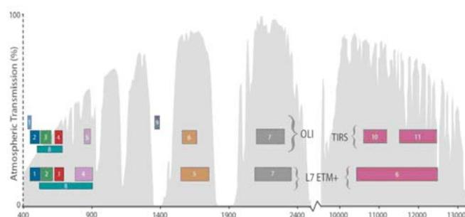
Fig. 1. Spectrum ranges of Landsat 7 and Landsat 8 channels
