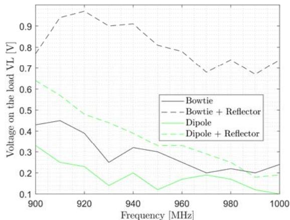
Fig.5. Voltage on the load, co-polarization.
