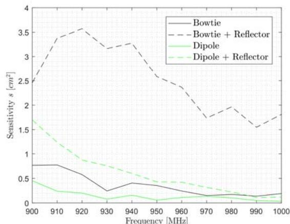
Fig.8. Sensibility  $s$  for the co-polarized case.
