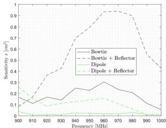
Fig.9. Sensibility  $s$  for the cross-polarized case.
