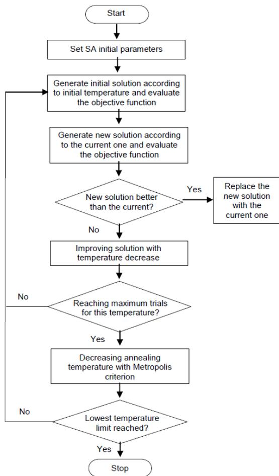
Fig.1. Simulated annealing algorithm flowchart
