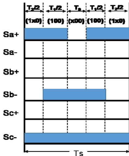
Fig.6. Switching pattern of the DSVPMOLSS method in sector 1
