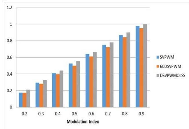
Fig.19. Normalized fundamental magnitude of load current over the modulation Index for SVPWM, 60DSVPWM and DSVPMOLSS methods
