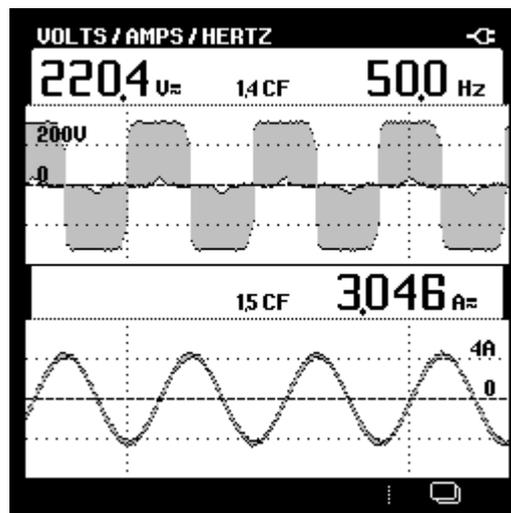
Fig.16. Line voltage and load current of the DSVPMOLSS method
