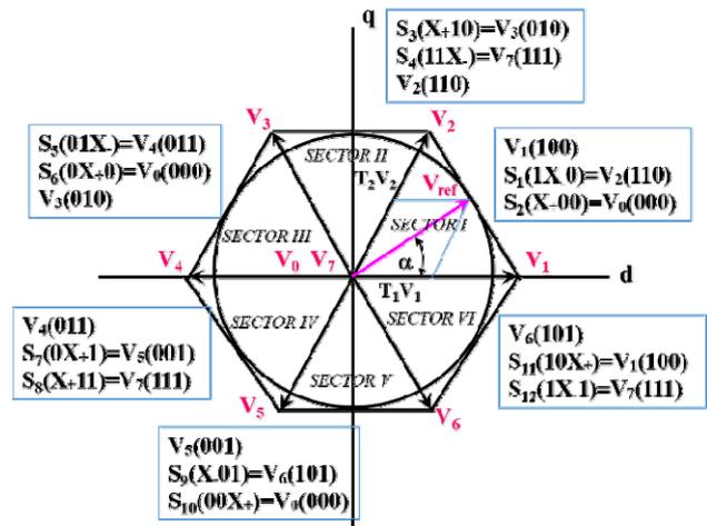
Fig.4. Voltage vectors of UPWM method
