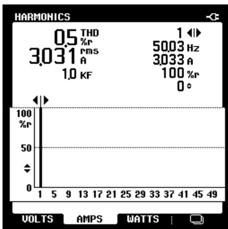
Fig.18. Magnitude spectrum of load current of the DSVPMOLSS method
