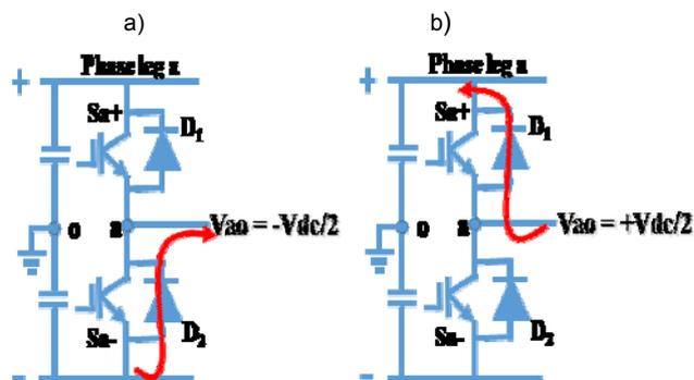
Fig.2. Output voltage at the a-leg; a) the state X<sub>-</sub> and b) the state X<sub>+</sub>.
