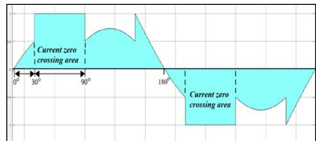
Fig.5. DPWM0 modulating waveform
