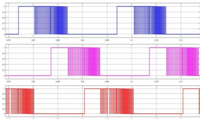
Fig.8. PWM signal of DSVPMOLSS
