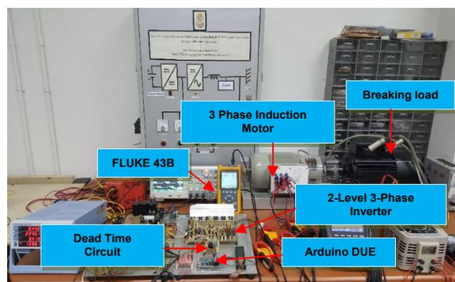
Fig.12. Experimental set-up
