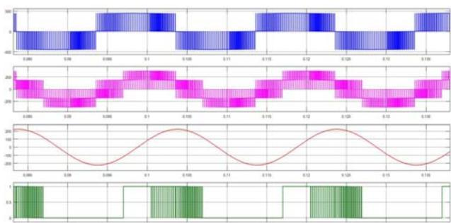
Fig.10. Line voltage ( $V_{AB}$ ), phase voltage ( $V_{AN}$ ), load current ( $I_A$ ) and PWM signal of upper switch ( $S_{a+}$ )
