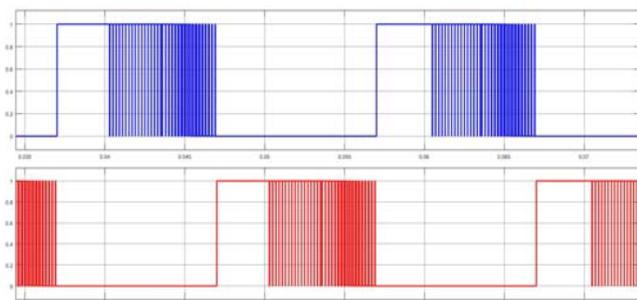
Fig.9. Upper and lower PWM signal of a leg
