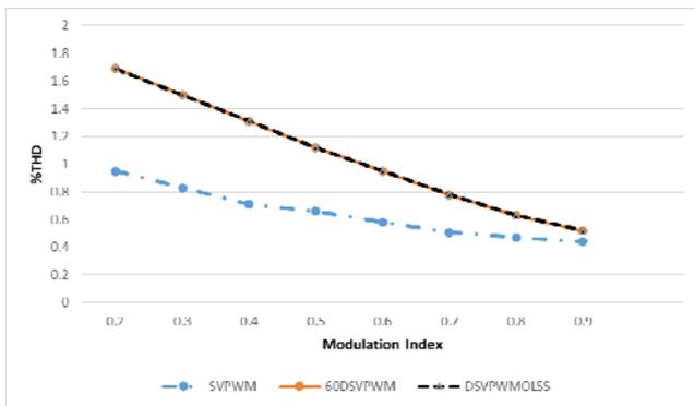
Fig.11. Simulation results (%THD vs. Modulation index) of SVPWM, 60DSVPWM and DSVPMOLSS at PF = 0.45 (lagging)
