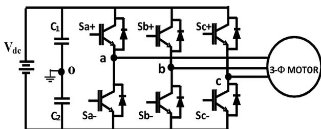
Fig.1. Two-level three-phase inverter
