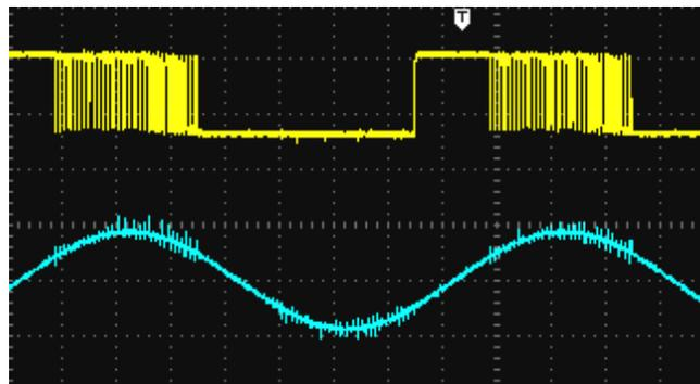
Fig.15. IGBT gate signals of lower switch ( $S_{a-}$ ) and load current (Horizontal axis: 2.5ms/div; Vertical axis: 10V/div and 4A/div)
