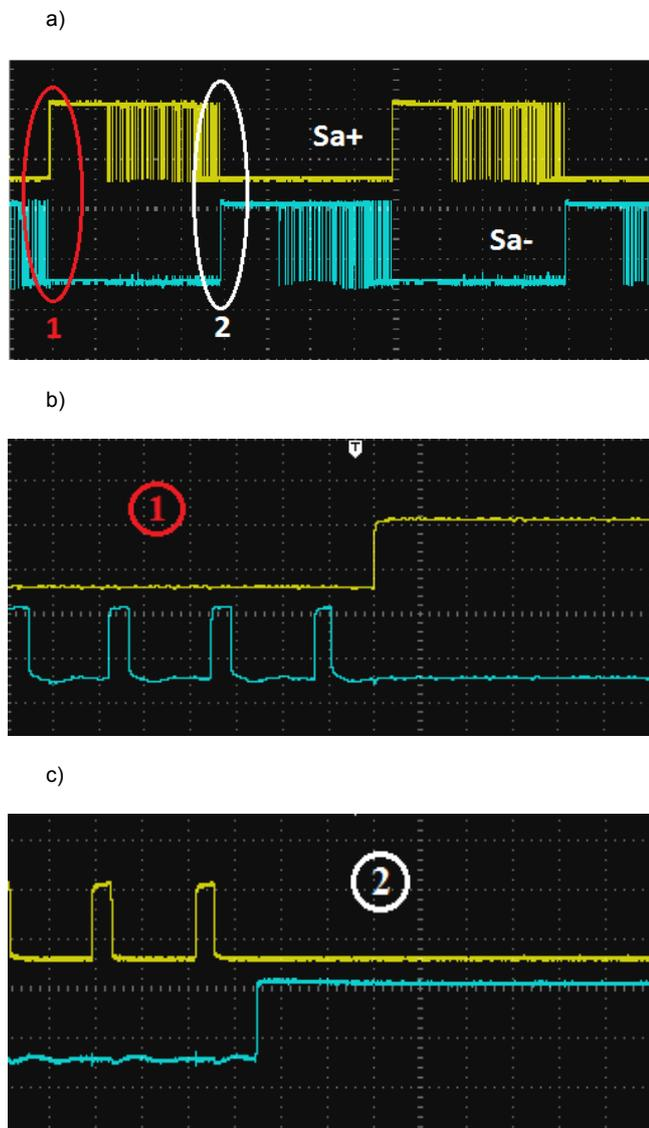
Fig.14. IGBT gate signals of upper and lower switches of the DSVPMOLSS method (Vertical axis: 10V/div; Horizontal axis: a) 2.5ms/div, b) and c) 100 $\mu$ s/div).
