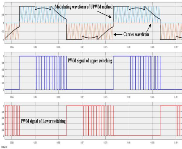
Fig.3. Carrier-based PWM of the UPWM method
