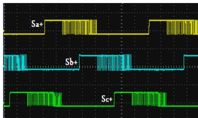
Fig.13. IGBT gate signals of three upper switches for the DSVPMOLSS method (Horizontal axis: 2.5ms/div; Vertical axis: 20V/div).
