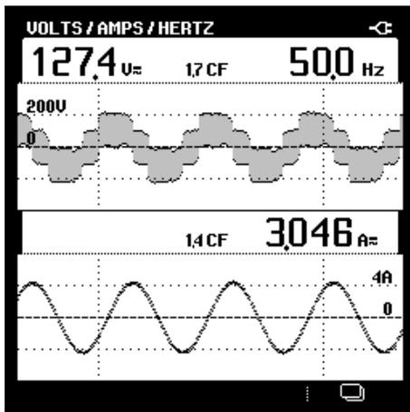
Fig.17. Phase voltage and load current of the DSVPMOLSS method
