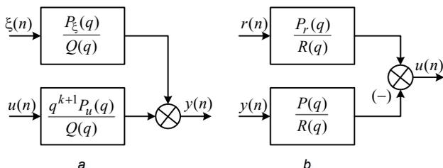
Fig. 1. Block diagrams of dynamic object (a) and control device (b)
