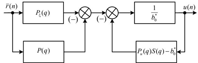
Fig.4. Block diagram of optimal restoring filter
