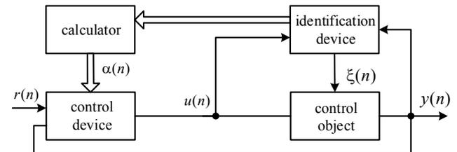
Fig.5. Block diagrams of indirect functional stable system
