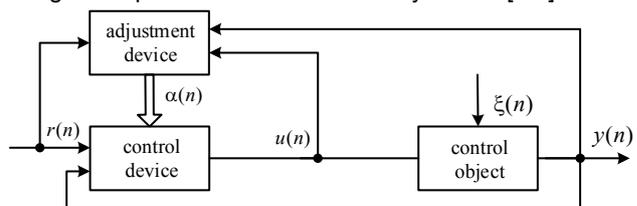
Fig.6. Block diagrams of direct functional stable system
