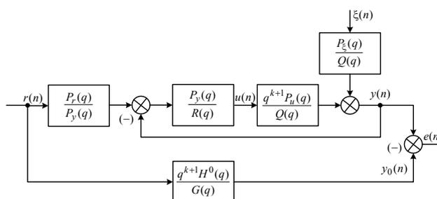
Fig. 3. Block diagram of optimal restoring device
