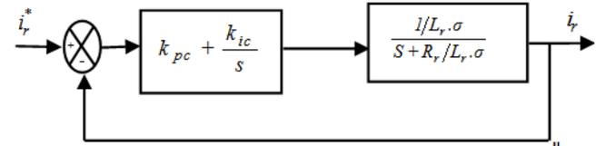
Fig.6. Closed loop for PI currents regulation
