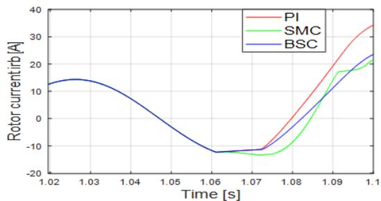
Fig.27. Rotor current  $i_{rb}$  under fault
