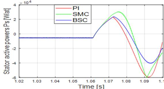
Fig.29. Measured stator active powers under fault
