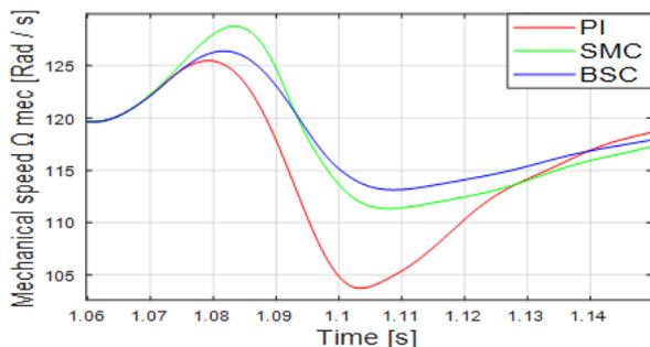
Fig.37. DFIG rotor mechanical speed under fault
