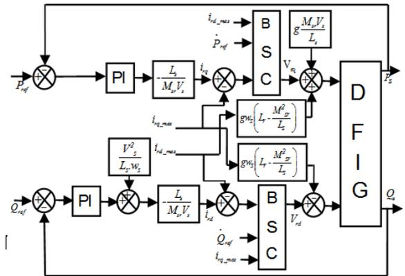
Fig.8. Block diagram of the hybrid BSC
