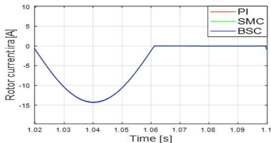
Fig.26. Rotor current  $i_{ra}$  under fault
