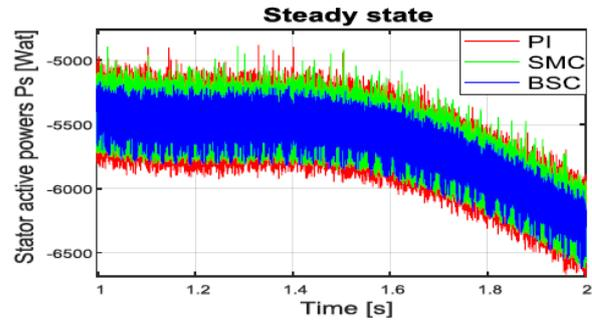
Fig.21. Measured stator active powers under steady state
