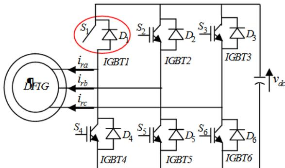
Fig.25. RSC during  $S_1$  switch open-circuit fault
