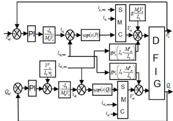
Fig.9. Block diagram of the hybrid SMC
