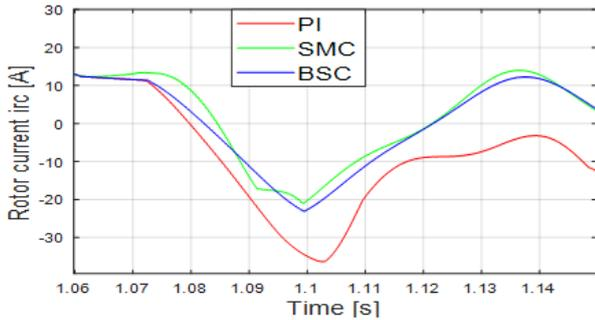
Fig.34. Rotor current  $i_{rc}$  under fault
