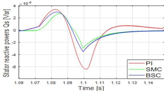
Fig.36. Measured stator reactive powers under fault
