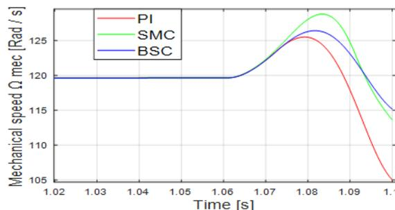
Fig.31. DFIG rotor mechanical speed under fault
