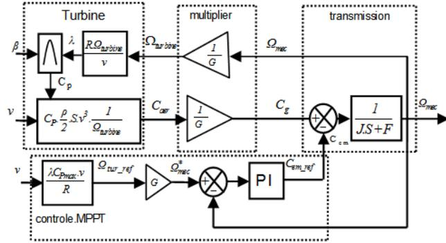
Fig.3. Block diagram of the turbine model With MPPT Control
