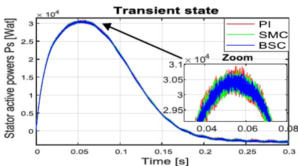
Fig.20. Measured stator active powers under transient state
