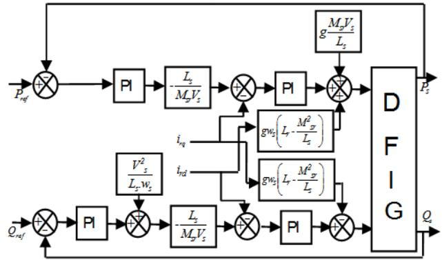
Fig.5. Block diagram of the PI indirect control with power loop
