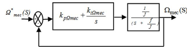
Fig.4. Closed loop for PI speed regulation
