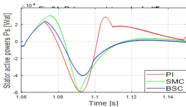
Fig.35. Measured stator active powers under fault
