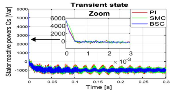
Fig.23. Measured stator reactive powers under transient state
