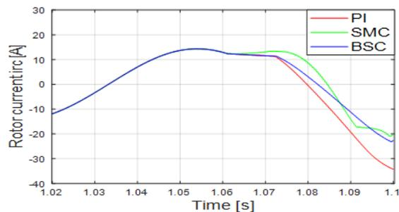
Fig.28. Rotor current  $i_{rc}$  under fault
