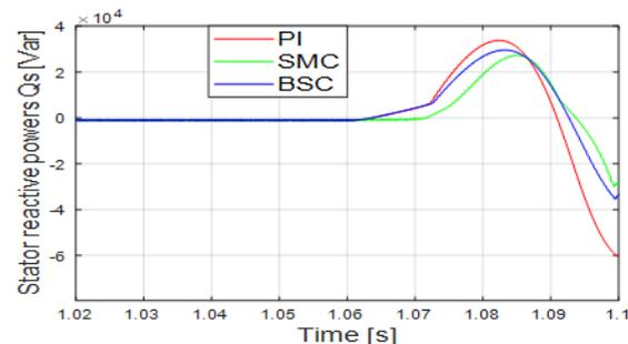
Fig.30. Measured stator reactive powers under fault
