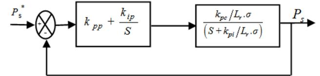
Fig.7. Closed loop for PI powers regulation
