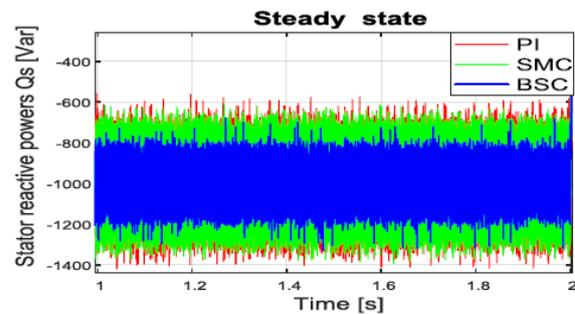
Fig.24. Measured stator reactive powers under steady state
