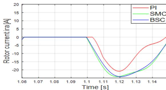
Fig.32. Rotor current  $i_{ra}$  under fault
