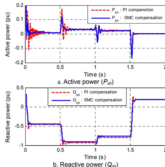
Fig.9. Active and reactive power after PI and SMC compensation
