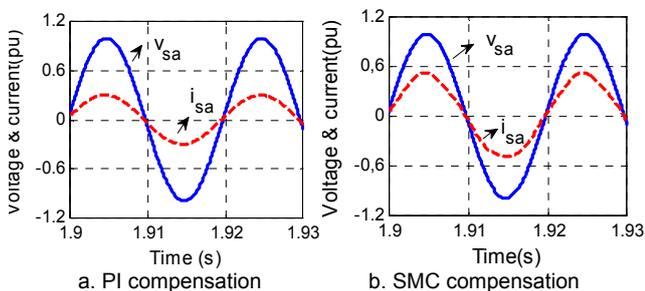
Fig.12. Grid voltage  $v_s$  and current  $i_s$  after compensation
