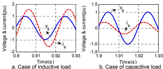
Fig.7. Grid voltage  $v_s$  and current  $i_s$  before compensation
