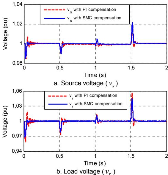
Fig.10. Source voltage  $v_s$  and load voltage  $v_r$  after PI and SMC compensation
