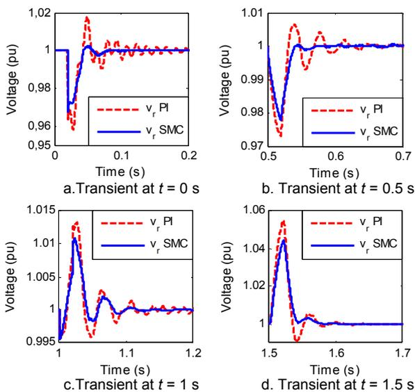
Fig.11. Transients of load voltage  $v_r$  for both PI and SMC compensations
