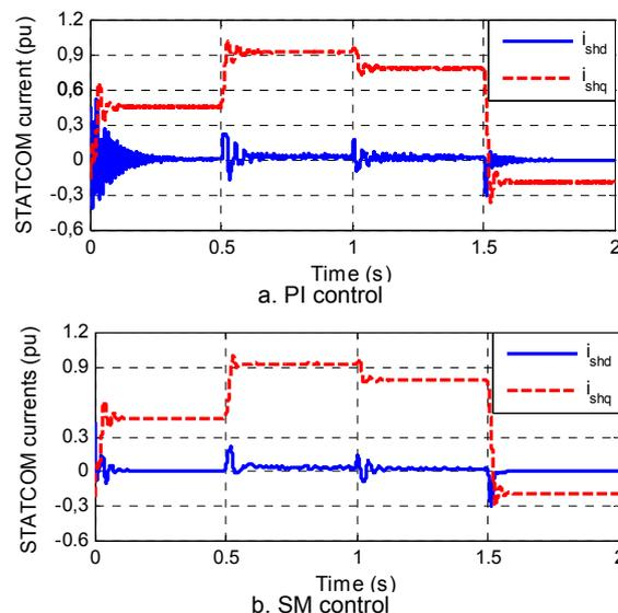
Fig.8. STATCOM currents  $i_{shd}$  and  $i_{shq}$  after compensation
