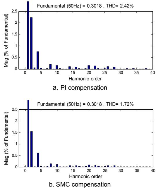
Fig.13. Harmonic spectrum of the source current  $i_s$
