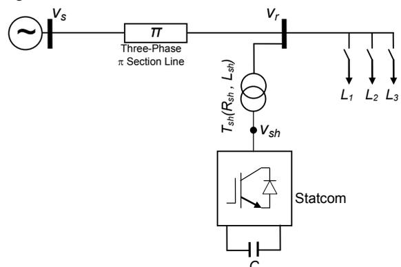
Fig.5. Single-line diagram of the studied network
