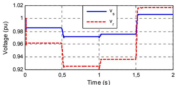
Fig.6. Source voltage  $v_s$  and load voltage  $v_r$  before compensation
