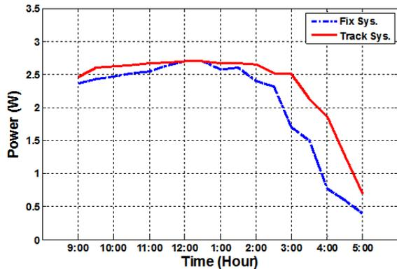
Fig. 8. Power vs. time with fixed and dual-tracking system
