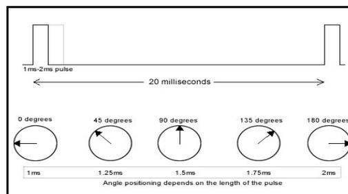
Fig. 4. Servo motor PWM timing diagram
