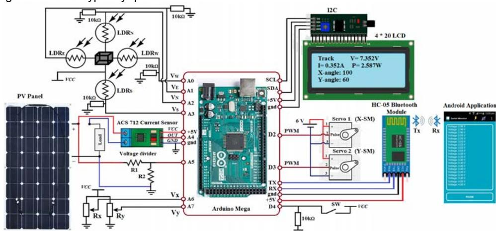
Fig.1. Block diagram of the proposed solar system
