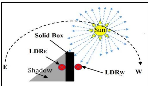
Fig. 2. Solar tracking under various positions of sun
