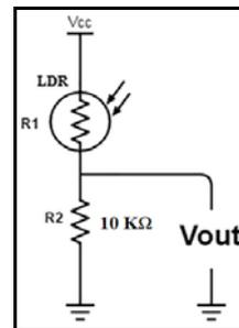
Fig. 3. Light intensity measuring circuit
