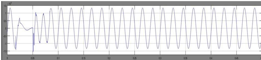
Fig. 9 Changing the voltage curve as a result of voltage supply to the PV plant bus in sHPP
