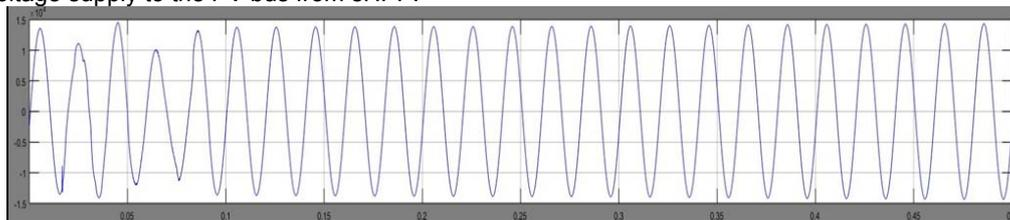
Fig. 8. Changing the voltage curve as a result of the parallel operation of the PV plant and sHPP with the electric network
