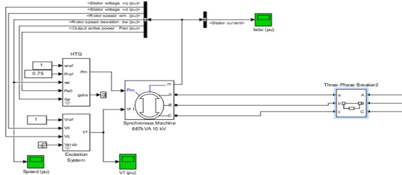
Fig. 7. Simulink model of Galjbievska small hydropowerplant which situated on the 999 bus
