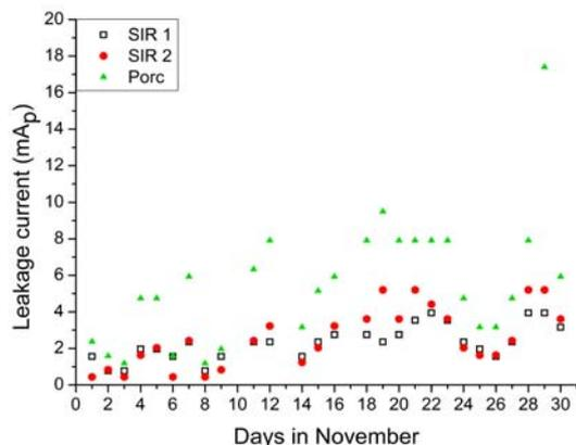
Fig. 4. Daily maximum leakage currents in November
