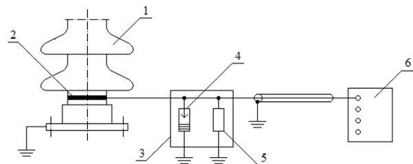
Fig. 2. A Schematic representation of the current measuring system.
