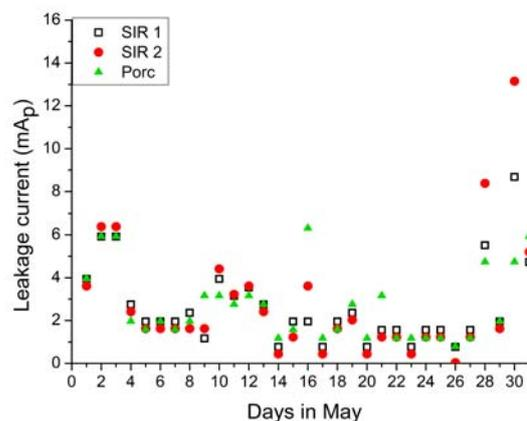
Fig.5. Daily maximum leakage currents in May
