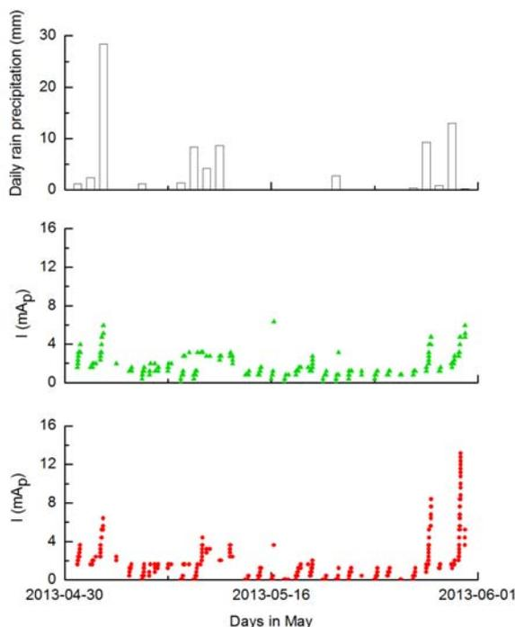
Fig.6. Current records and daily rain precipitation in May
