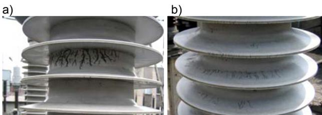
Fig.1. Surface erosion on shank (a) and on sheds (b) of silicone rubber
