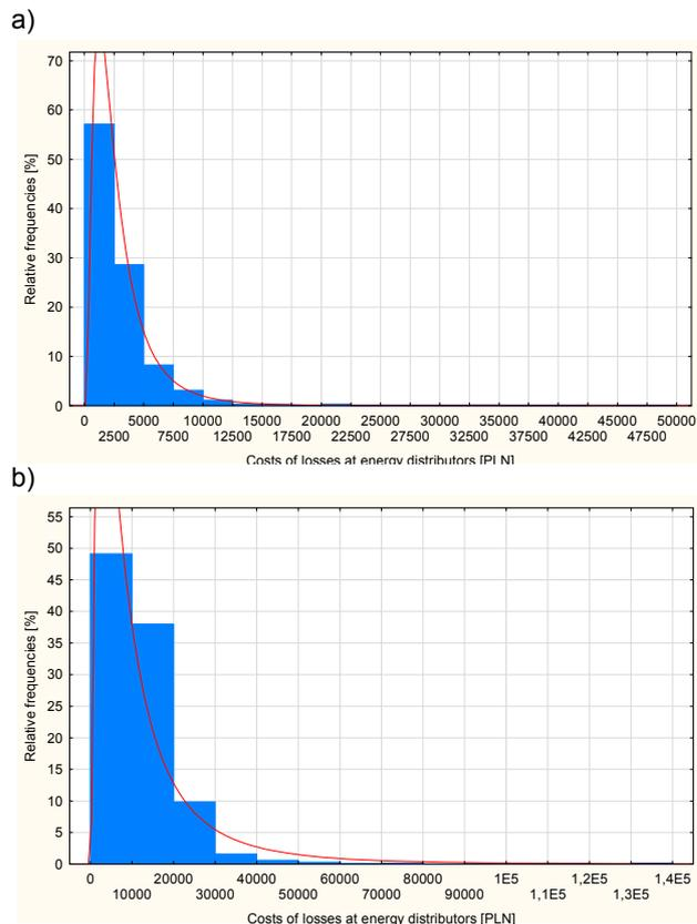
Fig. 6. Empirical and theoretical functions of probability density of costs of losses at energy distributors in case of failure of: a) MV overhead lines, b) MV cable lines
