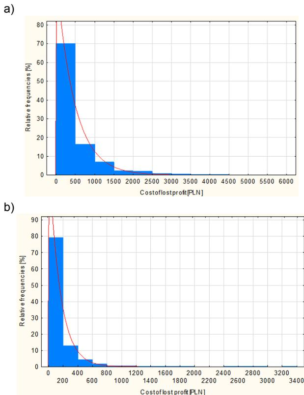
Fig. 5. Empirical and theoretical functions of probability density of lost profit costs in case of failure of: a) MV overhead lines, b) MV cable lines
