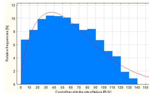
Fig. 4. Empirical and theoretical functions of probability of costs of travel to the site of failure in case of failure removal of: a) MV overhead lines, b) MV cable lines
