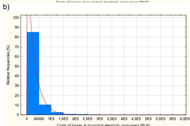
Fig. 7. Empirical and theoretical functions of probability density of costs of losses at energy consumers in case of failure of: a) MV overhead lines, b) MV cable lines
