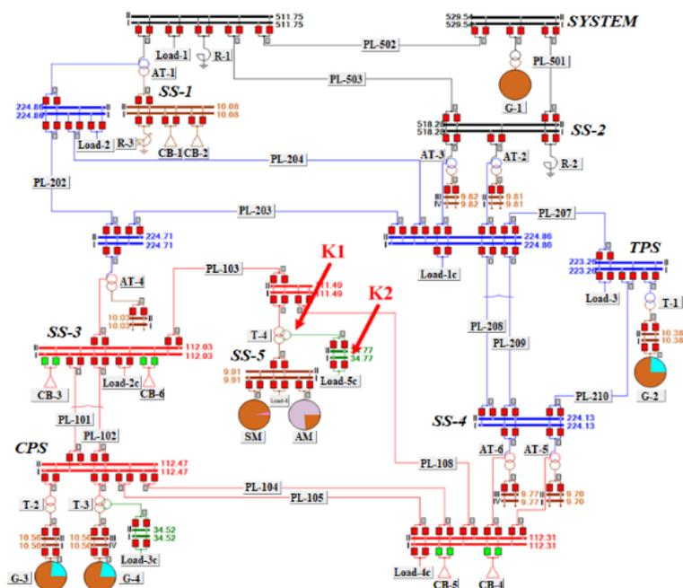
Fig.4. The Single-phase view of the simulated test EPS scheme in HRTSim, where G - generators; SM - synchronous motor; AM - asynchronous motor; PL - power transmission lines; AT - autotransformers; T - transformers
