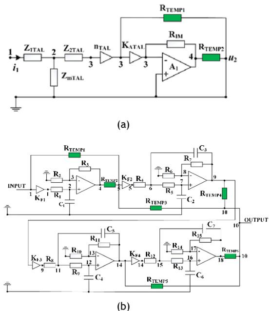
Fig.3. a) Universal equivalent scheme of ACT; b) Universal equivalent scheme of Butterworth LPF
