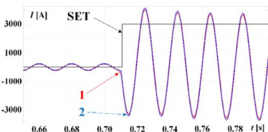
Fig.6. The oscillogram of the input signal in case of ABCG (point K1): 1 – recorded by the RP terminal, 2 – the original signal, recorded in COMTRADE
