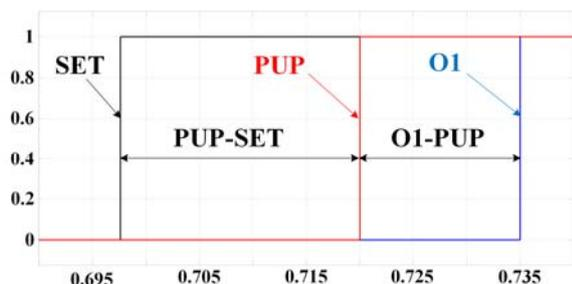
Fig.7. Logic signals in case of ABCG (point K1): O1 – tripping of the RP terminal output relay; PUP – tripping command of the microprocessor; SET – tripping of the 'ideal' protection (without internal delays)
