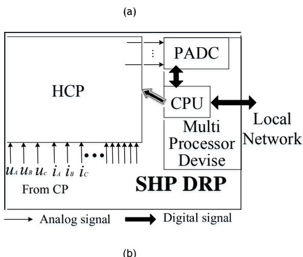
Fig.1. a) The external view of specialized hybrid processor for DRP simulation; b) Structural scheme SHP DRP
