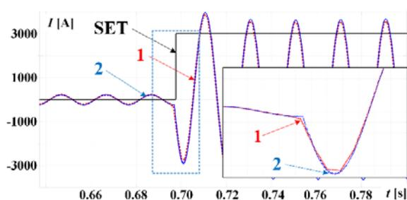
Fig.5. The oscillogram of the input signal in case of ABCG (point K1): 1 – recorded by the RP terminal, 2 – the original signal, recorded in COMTRADE
