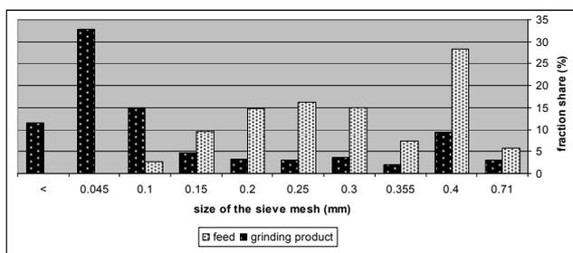
Fig. 5. Grit size distribution before and after grinding in an electromagnetic mill (quartz sand)
