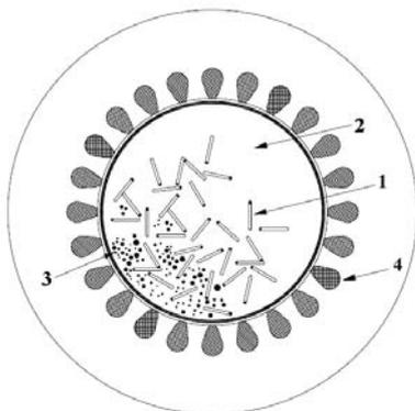
Fig. 1. Electromagnetic mill with latent poles [9]: 1 – grinding media, 2 – working chamber, 3 – material ground, 4 – winding in grooves
