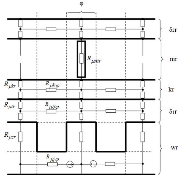
Fig. 3. Developed magnetic circuit of the mill (without proportion): wr – inductor area,  $\delta_r$  – air gap area, kr – working chamber area, mr – area of the grinding media,  $\phi$  – area analysed
