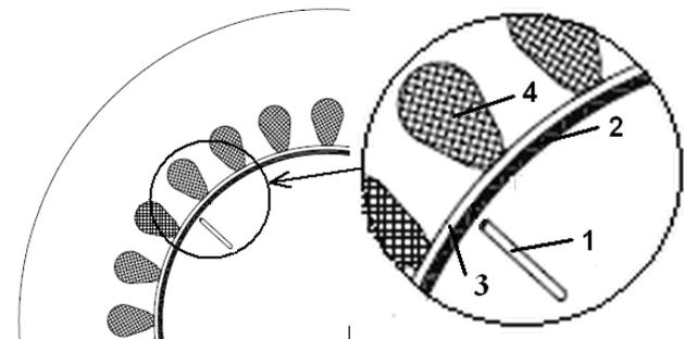
Fig. 2. Fragment of the area analysed: 1 – grinding media (mr – millennium area), 2 – working chamber 1 mm (kr – working chamber area), 3 – air gap 1,5 mm (δr – air gap area), 4 – nursery with windings (rr – inductor area)
