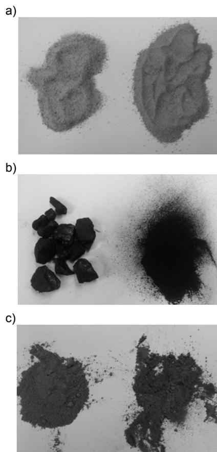
Fig. 4. Raw material before (on the left) and after (on the right) grinding: (a) quartz sand, (b) hard coal, (c) volatile dust
