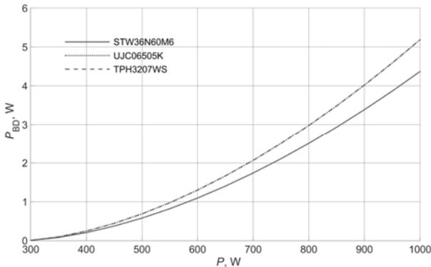
Fig. 7. Calculated freewheeling diode conduction loss in a single transistor as a function of output power of the converter at a switching frequency of 300 kHz.
