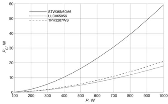
Fig. 4. Calculated conduction loss in a single transistor as a function of output power of the converter at a switching frequency of 300 kHz and junction temperature of 150°C
