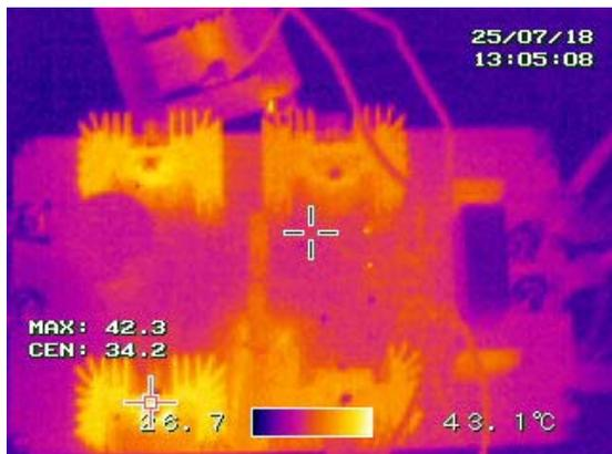
Fig. 15. Infrared photograph of the converter with TPH3207WS gallium nitride transistors at the nominal output power
