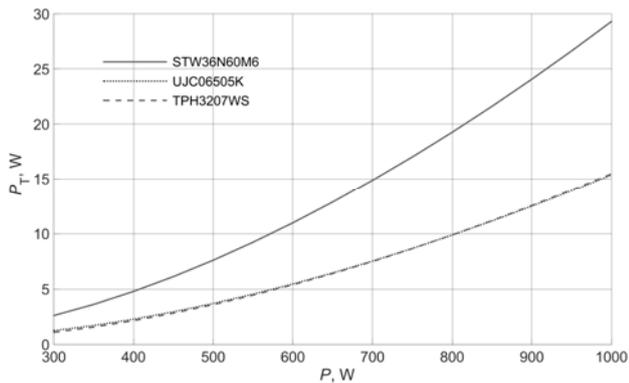
Fig. 9. Calculated total power loss in a single transistor as a function of output power of the converter at a switching frequency of 300 kHz and junction temperature of 25°C
