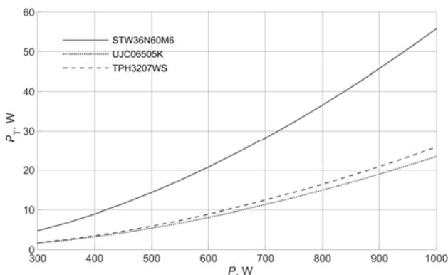
Fig. 12. Calculated total power loss in a single transistor as a function of output power of the converter at a switching frequency of 500 kHz and junction temperature of 150°C
