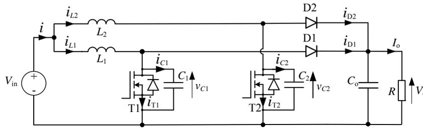
Fig. 1. Topology of the examined converter
