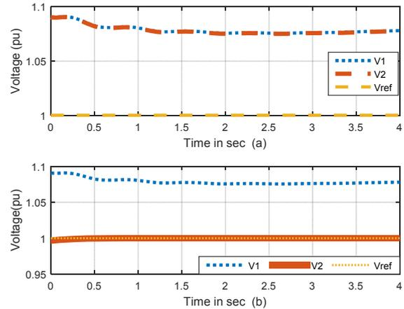
Fig.10. Voltage regulation a. Without SVC, b. With SVC
