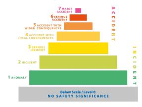
Fig. 2. INES scale according to IAEA [5]
