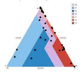
Fig. 5. Defects recognized by the Duval triangle method for data came from transformers in which partial discharges were found.
