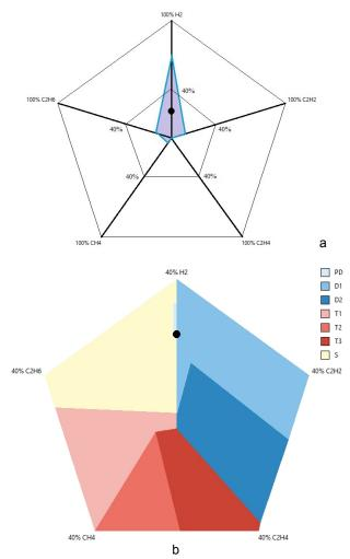
Fig. 3. Location of the defect in the Duval pentagon method
