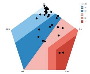
Fig. 6. Defects recognized by the Mansour pentagon method for data came from transformers in which partial discharges were found.
