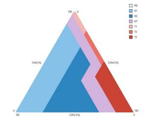
Fig. 2. Location of defect zones in the basic variant of the Duval triangle
