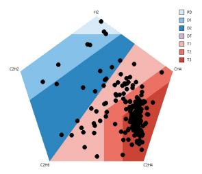
Fig. 8. Defects recognized by the Mansour pentagon method for data came from transformers in which thermal faults were found.
