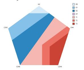
Fig. 4. Location of defect zones in the Mansour pentagon.
