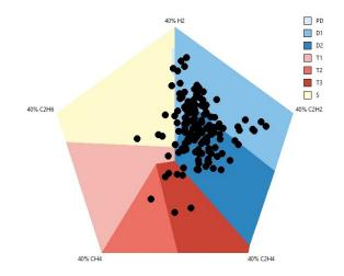
Fig. 7. Defects recognized by the Duval pentagon method for data came from transformers in which discharges were found.
