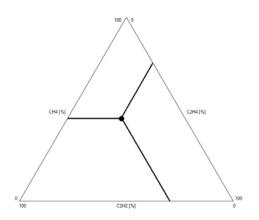
Fig. 1. The method of determining the position of a point inside a Duval triangle based on the coordinates  $\%C_2H_2,\,\%CH_4$  and  $\%C_2H_4$
