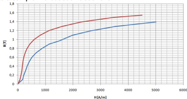
Fig. 2. DC magnetization curves of Kovar: without special treatment – red line, and after complex thermal-mechanical treatment – blue line
