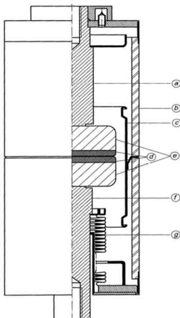
Fig. 1. Cross section of a vacuum interrupter: (a) fixed contact stem, (b) ceramic or glass insulator, (c) vapour condensation shield, (d) copper-tungsten contacts, (e) contacts, (f) moving contact stem, (g) bellow
