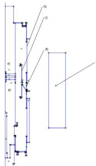
Fig. 3. Cross section of a vacuum interrupter: (a) a fixed contact stem, (b) a ceramic or glass insulator, (c) vapour condensation shield, (d) housing sleeve with flanges, (e) magnet coil
