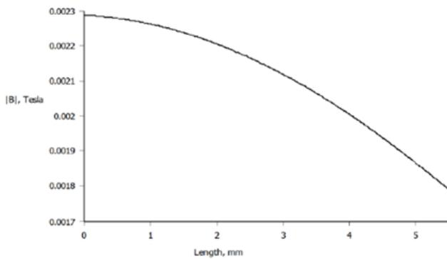
Fig.5. Magnitude of magnetic flux density between contacts with a shield made of Kovar without a special treatment, as a function of distance from centre of a chamber
