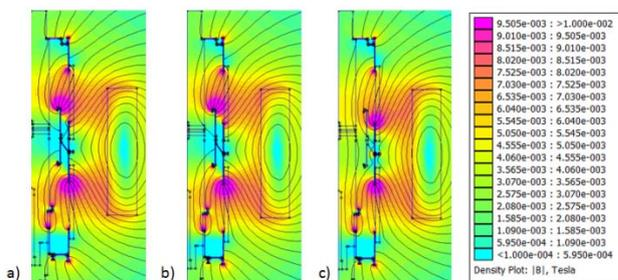
Fig. 4. Magnetic flux density distribution and magnetic flux lines for simulations: (a) with Kovar without special treatment shield, (b) with Kovar with complex thermal-mechanical treatment shield and (c) with copper shield
