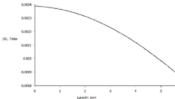
Fig.6. Magnitude of magnetic flux density between contacts with a shield made of Kovar after a special treatment, as a function of distance from centre of a chamber
