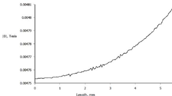
Fig.7. Magnitude of magnetic flux density between contacts with a shield made of copper, as a function of distance from centre of a chamber
