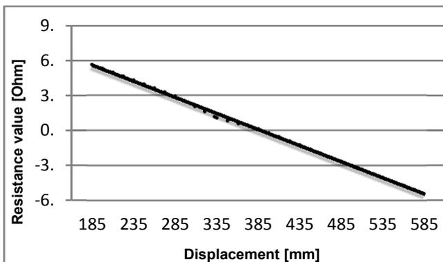
Fig. 5. The occurring resistances during piston displacement
