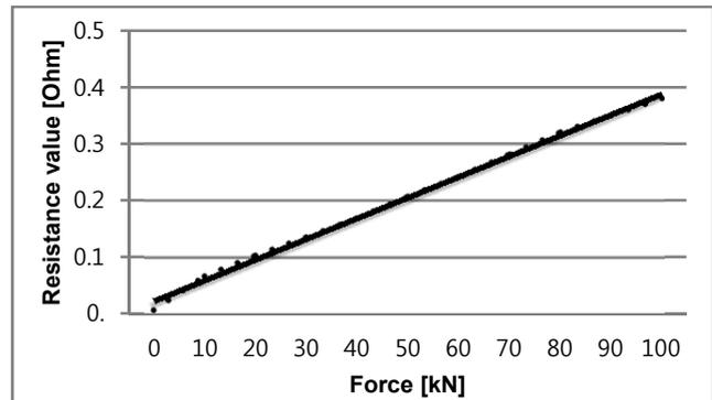
Fig. 4. the measured resistances caused by the piston force
