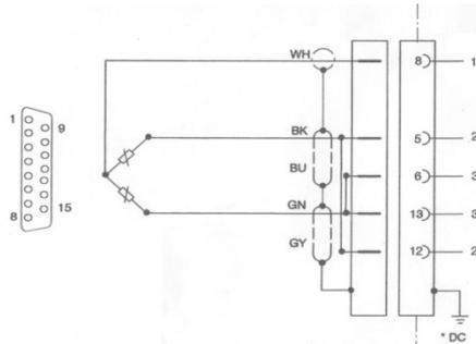
Fig. 2. The schematic of the tensometers half-bridge set used in measurements: 1) Measured signal, 2, 3) Voltage excitation bridge, 2', 3') Read
