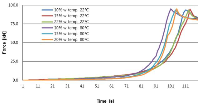
Fig 6. The mean course of the pressure value caused by the piston path during the compaction process of the shredded forest residues
