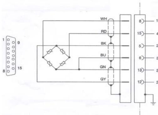
Fig. 3. The schematic of the tensometers bridge set used in measurements: 1) Measured signal, 2, 3) Voltage excitation bridge, 2', 3') Read
