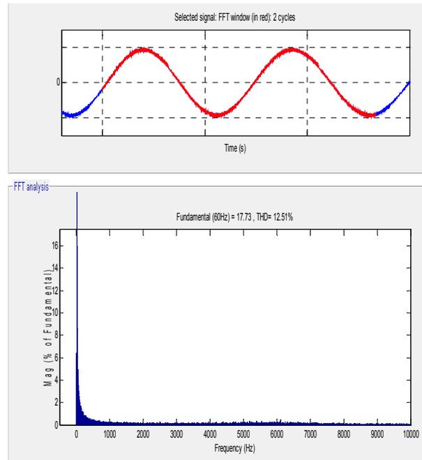
Fig. 7. Spectrum of current (DTC conventional)
