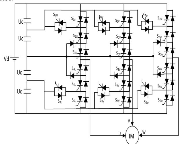
Fig. 1. Schematic diagram of a five-level GTO inverter
