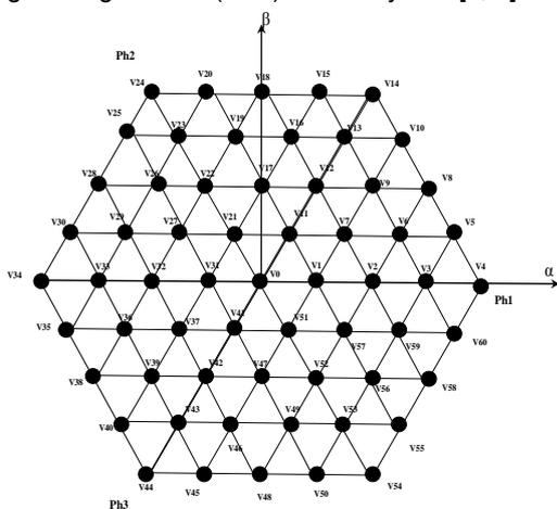
Fig. 2. Topography of the 61 vectors generated by a NPC structured five-level inverter
