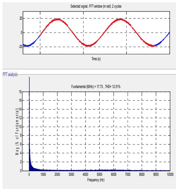
Fig. 9. Spectrum of current (DTC based fuzzy logic)
