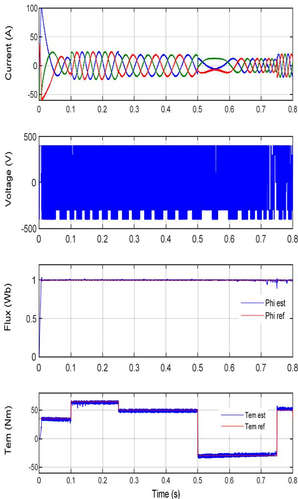
Fig. 8. Simulations results of DTC based Fuzzy logic controllers
