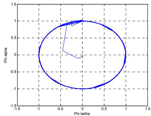
Fig. 10. Stator Flux Trajectory (classical DTC)
