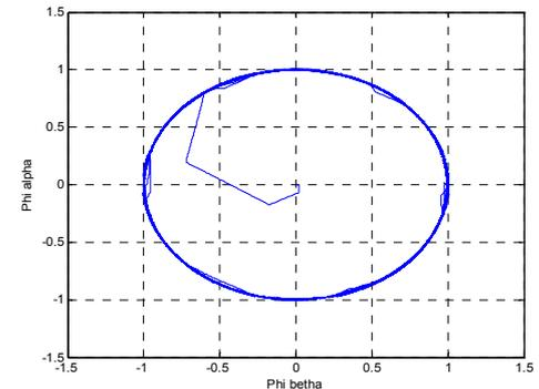
Fig. 10. Stator Flux Trajectory (DTC based fuzzy logic)
