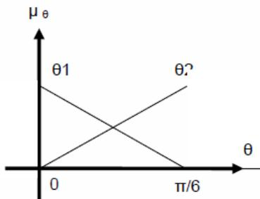
Fig. 4. New member for flux vector position.
