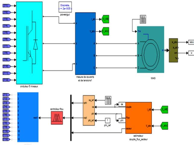
Fig. 5. The structure of the simulation model of proposed DTC based fuzzy logic control
