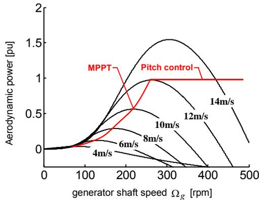
Fig.4. Aerodynamic powers various speed characteristics with tracking curve
