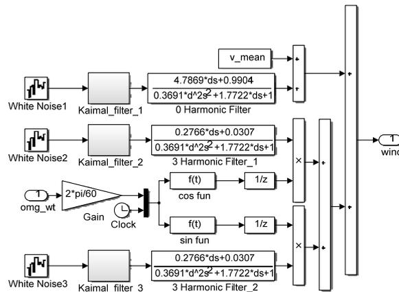
Fig.2. FAST Simulink implementation of aerodynamic wind speed model
