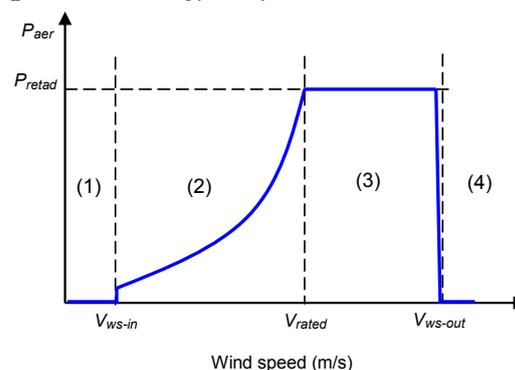
Fig.1. Areas of operation and control WECS
