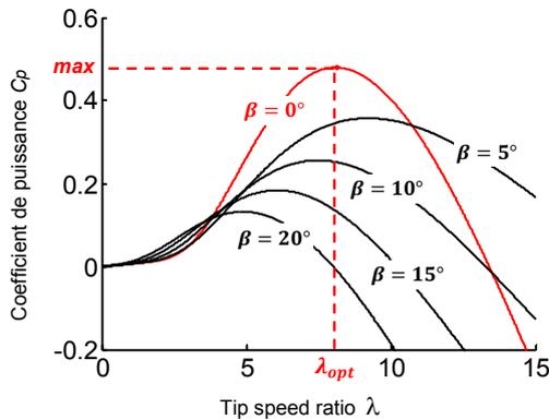
Fig.3. Power coefficient variation against TSR and different pitch angle
