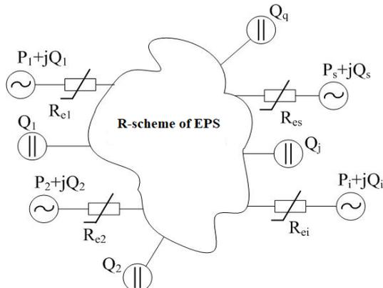
Fig. 5. The circuit diagram of the electric network with economic supports
