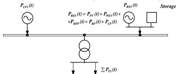
Fig. 1. Power supply balance in the electric grid
