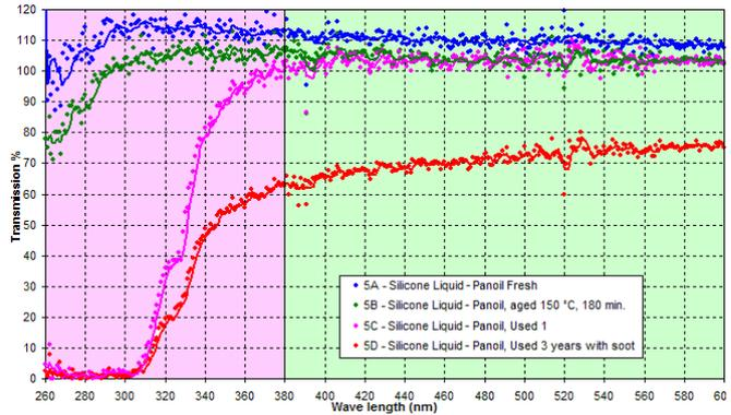
Fig.9. Differences in Spectral Trans. for Different Degradations
