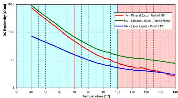
Fig.3. DC Resistivity of Liquid Samples
