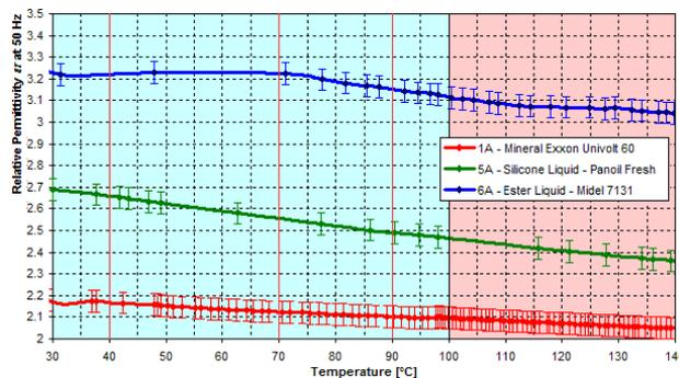
Fig.4. Relative Permittivity of Liquid Samples
