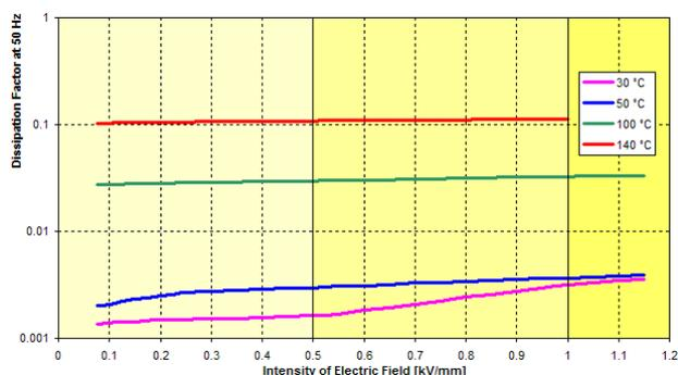
Fig.6. Dependence of Dissipation Factor of Mineral Exxon Oil on Intensity of Electric Field and Temperature
