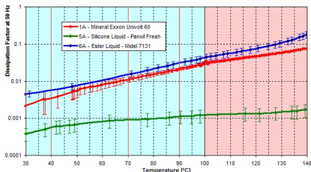
Fig.5. Measured Dissipation Factor of Oil and Liquid Samples
