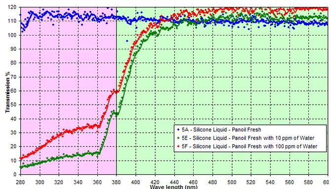
Fig.10. Spectral Trans. of Silicone Liquids with Water Content
