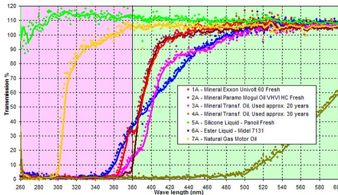
Fig.8. Differences in Spectral Trans. for Different Types of Liquids
