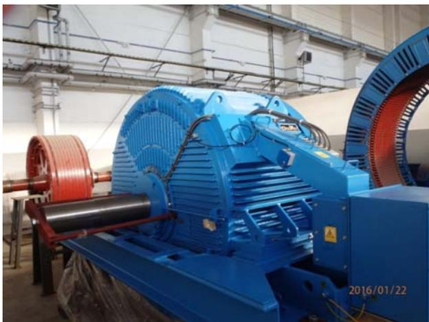
Fig. 8. View of the synchronous motor with permanent SMH type magnets
