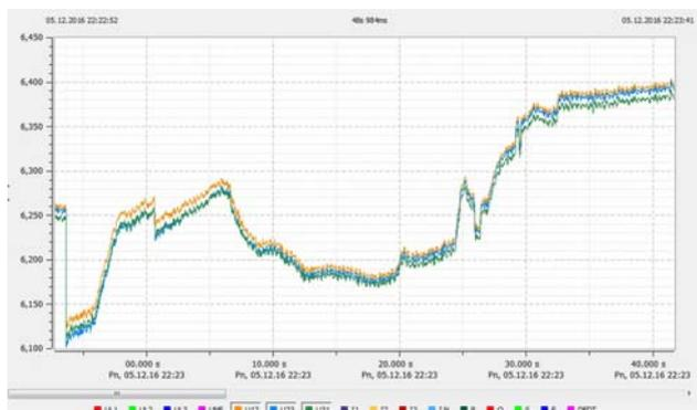
Fig. 3. Time waveforms of the effective value of phase-to-phase voltages during the start-up of the SAS-type motor with a resistor starter
