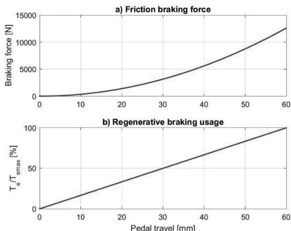
Fig. 11. a) Frictional braking force vs brake pedal position; b) Degree of utilization of the electric braking (ratio of the torque actually generated by the electric machine to the maximum braking torque obtainable from the machine at a specific operating point)
