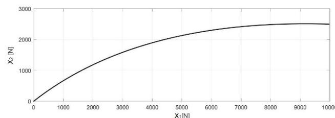
Fig. 3. Ideal braking force distribution curve (“l-curve”) plotted for the data specified in Table 1.
