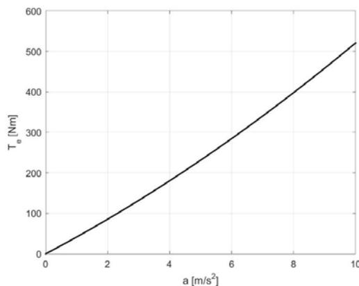
Fig. 5. Electric machine braking torque vs braking deceleration
