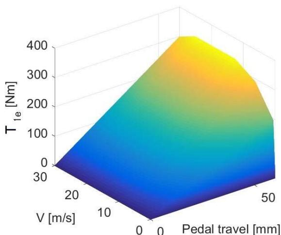
Fig. 12. Regenerative braking torque as a function of brake pedal position and vehicle speed
