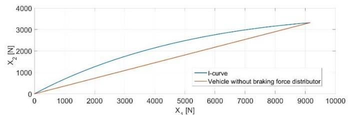
Fig. 9. Ideal braking force distribution curve (I-curve) and distribution of braking forces for a vehicle with no braking force regulator
