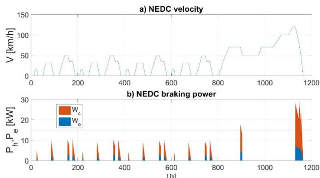
Fig. 13. a) Time history of vehicle speed in the NEDC test; b) Braking power division for the parallel braking in the NEDC test
