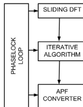
Fig. 1. Block diagram illustrating the iterative process of reference current detection for APF
