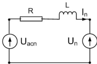
Fig. 13. Impedance and voltage drop for  $n$ -th harmonic
