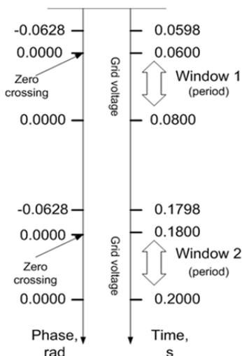
Fig. 9. Window synchronization-grid voltage processed
