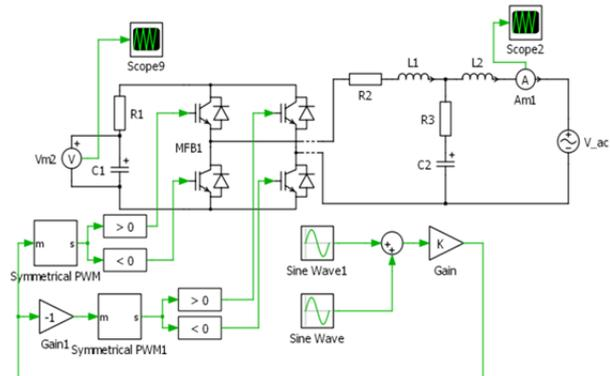
Fig. 14. PLECS model of the PWM inverter
