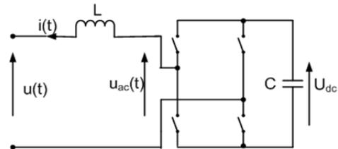
Fig. 12. Current source realization, DC/AC bipolar converter
