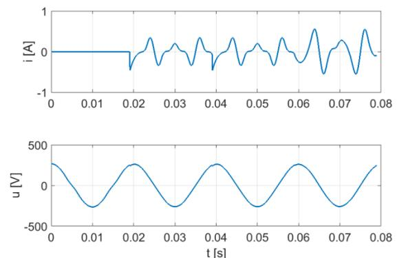
Fig. 19. Compensator current (upper waveform) and improved voltage (lower waveform) within compensating process
