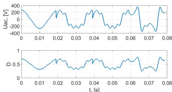
Fig. 20. DC/AC converter signals: ac voltage (upper drawing), b) duty ratio (lower drawing)
