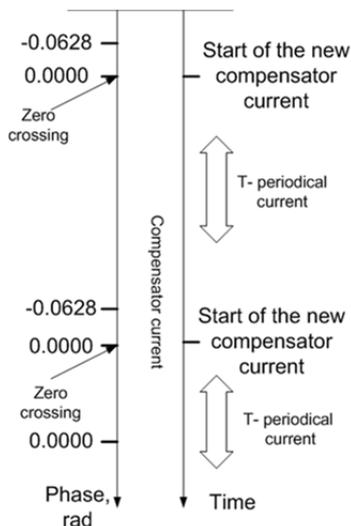
Fig. 11. Synchronization of compensator current intervals
