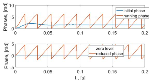
Fig. 8. Window synchronization-simulation waveforms.
