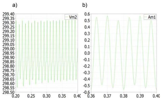
Fig. 16. Simulation waveforms for  $\delta = -0.00007$  a) capacitor voltage, b) compensator current (third harmonic)
