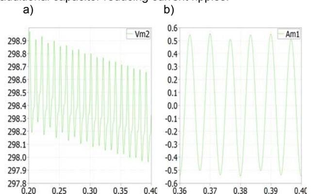
Fig. 15. Simulation waveforms for  $\delta = 0$  a) capacitor voltage, b) compensator current (third harmonic)
