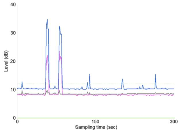
Fig. 5. Time chart of partial discharges activity – transmission tower no. 2, without rain
