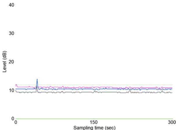
Fig. 4. Time chart of partial discharges activity – transmission tower no. 1, without rain
