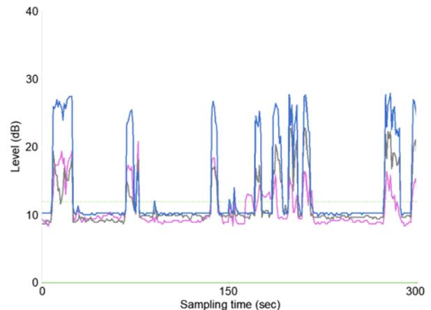
Fig. 6. Time chart of partial discharges activity – transmission tower no. 2, rainfall
