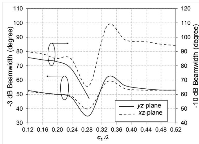
Fig.3. Simulated beamwidths of the OERW with FSCA for various length  $c_1$ .
