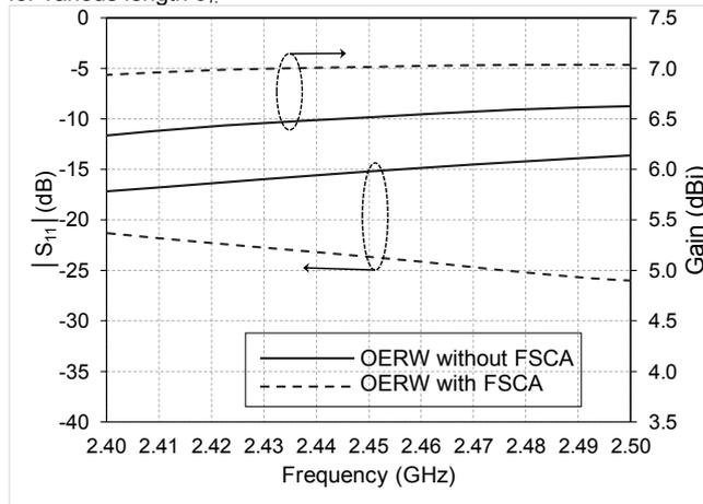
Fig.4. Simulated  $|S_{11}|$  and gain of the proposed antenna with and without FSCAs
