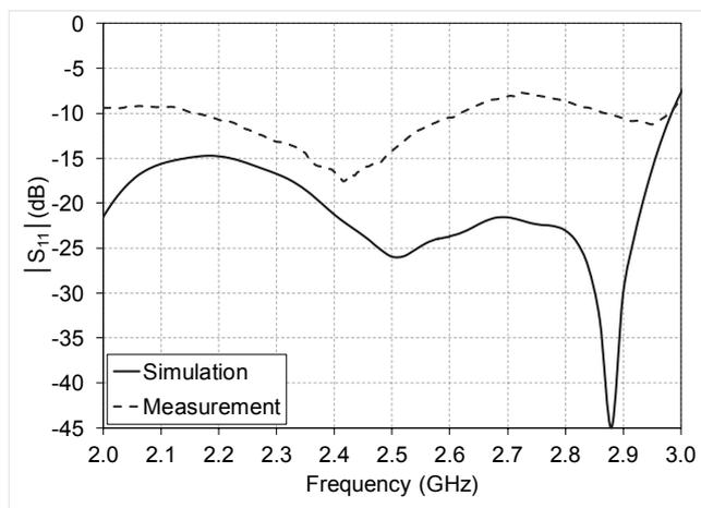
Fig.5. The simulated and measured  $S_{11}$  versus frequency
