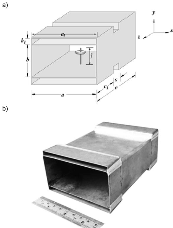
Fig.1. Geometry of the proposed antenna: (a) model and (b) prototype
