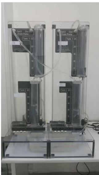
Fig. 1. Quanser's quadruple tanks system.
