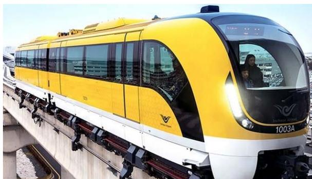
Fig. 10. Car body incorporates traditional Korean curvature and honeycomb pattern on both sides of the car (below windows).
