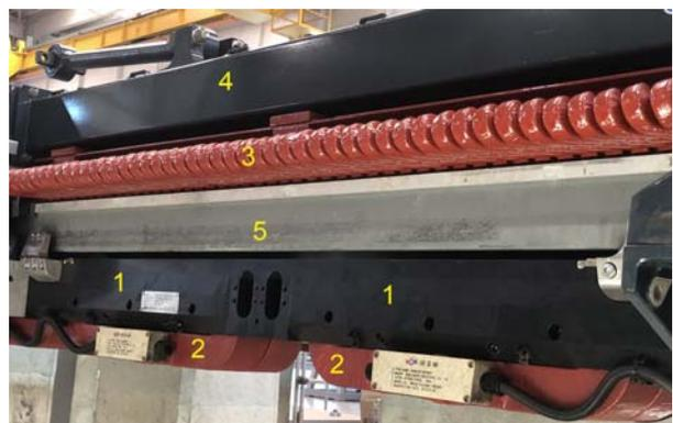
Fig. 7. Suspension electromagnets: 1 – steel core of the electromagnet, 2 – coil of the electromagnet, 3 – three-phase winding of the primary unit of the LIM, 4 – bogie of the car, 5 – steel reaction rail for suspension electromagnet (part 5 of Fig. 6). Photo taken in the maintenance depot.
