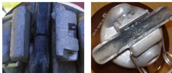
Fig. 2: Two examples of damages to insulation of covered conductor and conductor clamp.
