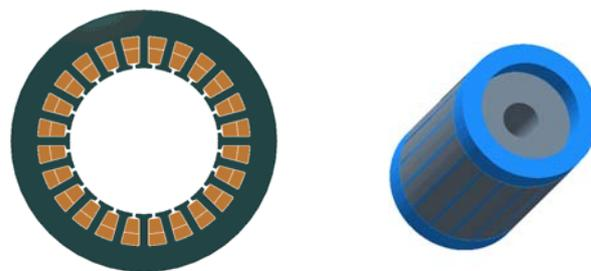
a) stator with windings                      b) squirrel cage rotor
