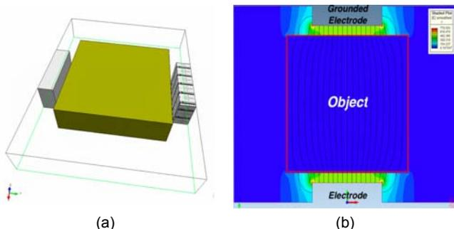
Fig.10. Capacitive sensor: 3D geometry (a), electric field map (b).
