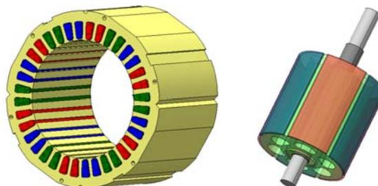
a) stator with windings                      b) rotor with PM
