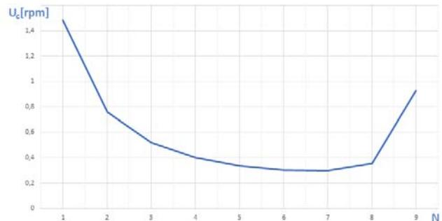
Figure 5 - total uncertainty  $U_c(\omega)$  versus N value after including the t-Student distribution for 1002 rpm speed measurement
