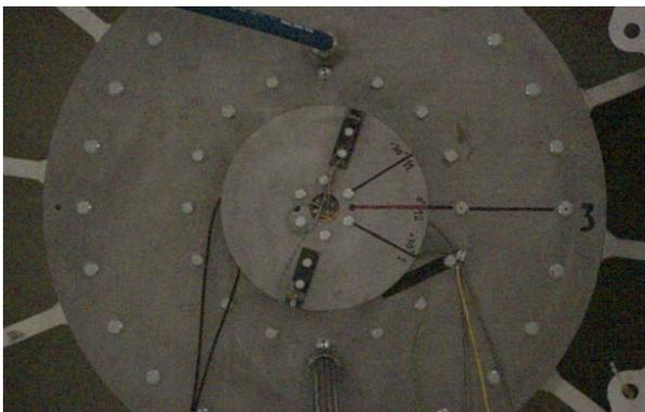
Figure 2 - image acquired by the high speed camera at the moment when markers on rotor and stator align
