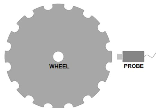
Fig. 1 - rotational speed measurement assembly
