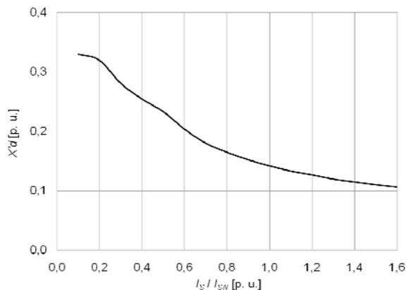
Fig. 11. Dependence transient reactance in direct axis on stator current
