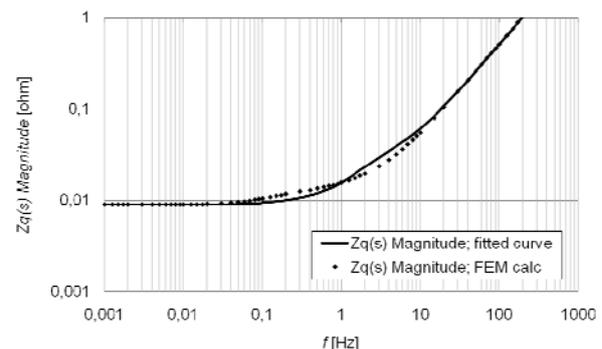
Fig. 6. Quadrature-axis magnitude impedance
