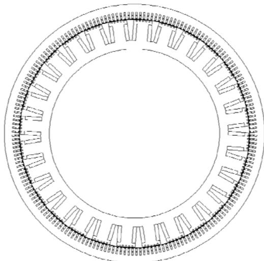
Fig. 1. Field model of investigated synchronous machine
