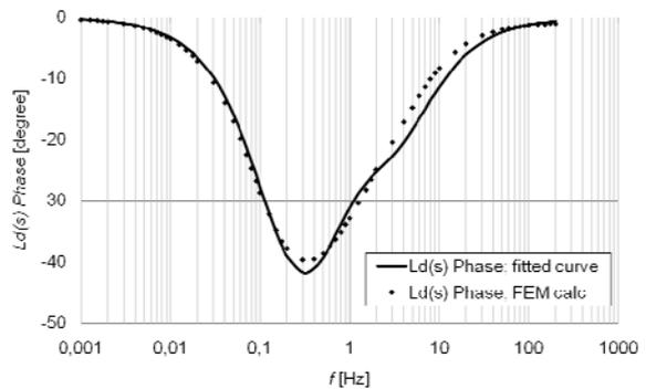
Fig. 5. Direct-axis phase inductance
