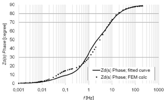
Fig. 3. Direct-axis phase impedance
