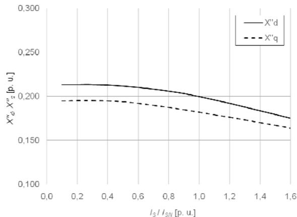
Fig. 12. Dependence sub-transient reactances in direct and quadrature axes on stator current
