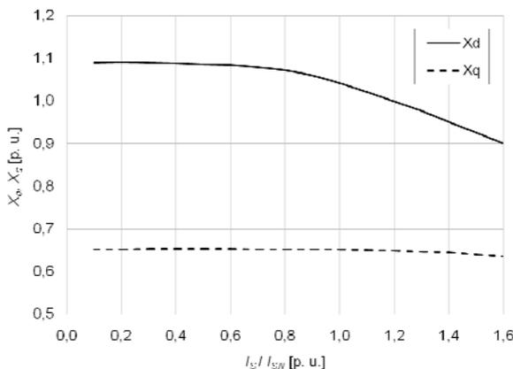
Fig. 10. Dependence synchronous reactances in direct and quadrature axes on stator current
