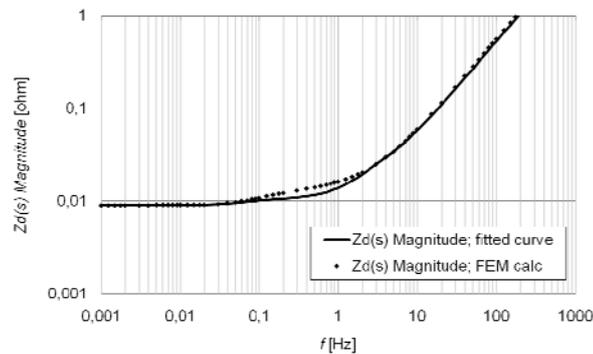
Fig. 2. Direct-axis magnitude impedance
