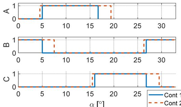
Fig. 5. Sequence of switching an SRM phase
