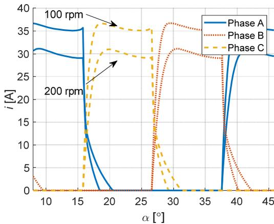
Fig. 7. Current waveforms in the SRM for Cont. 1
