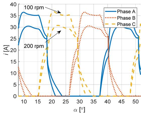
Fig. 9. Current waveforms in the SRM for Cont. 2
