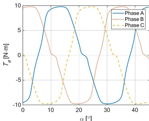
Fig. 2. Generated electromagnetic torque vs. rotor angle for each phase at a constant current value of  $I=35A$
