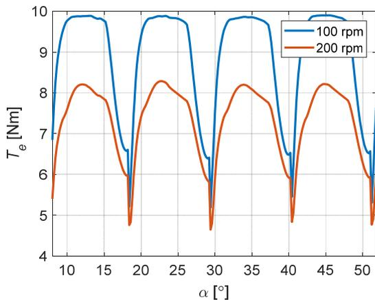
Fig. 8. Electromagnetic torque generated by the SRM when control is Cont. 2
