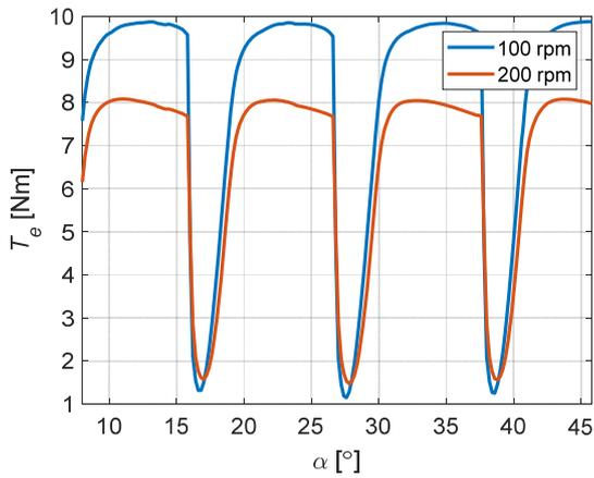
Fig. 6. Electromagnetic torque generated by the SRM when control is Cont. 1
