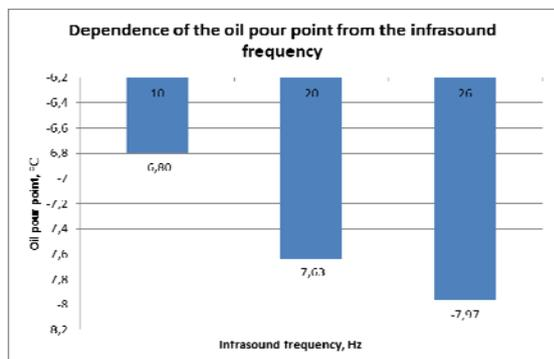
Fig.2. The diagram of the dependence of the oil pour point on the infrasound frequency
