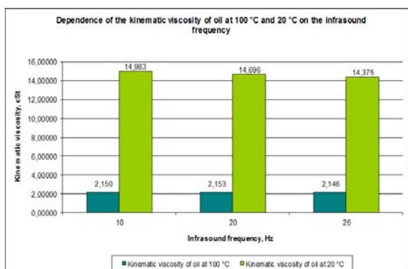
Fig.4. The diagram of the dependence of the kinematic viscosity of oil at 100 °C and 20 °C on the infrasound frequency
