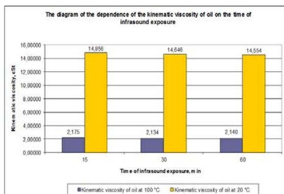
Fig.5. The diagram of the dependence of the kinematic viscosity of oil on the time of infrasound exposure
