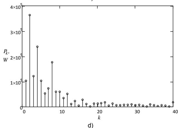
Fig. 1. The results of the analysis of the energy processes and the quality of the electric energy of the influencing consumer of the subscriber: a) the consumed voltage and current curves; b) the instantaneous power components; c) the frequency spectra of the consumed current; d) the frequency spectra of the power
