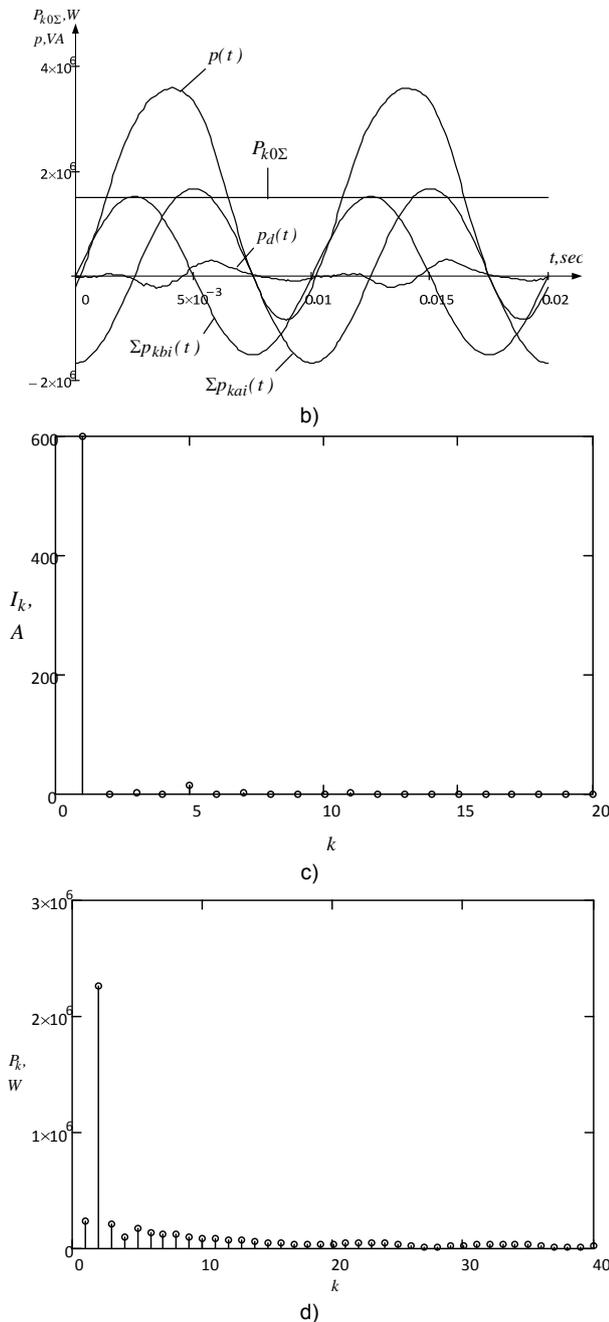
Fig. 2. The results of the analysis of the energy processes and the quality of the electric energy at the enterprise internal input: a) the consumed voltage and current curves; b) the instantaneous power components; c) the frequency spectra of the consumed current; d) the frequency spectra of the power
